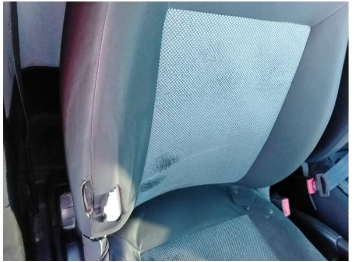
6: Seat Back Cover osf Torn Over 3mm
