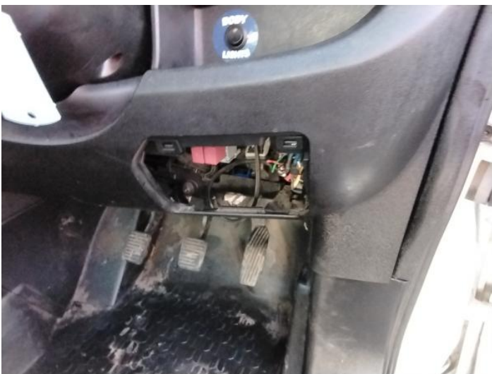
7: Fascia Panel Missing Replace
