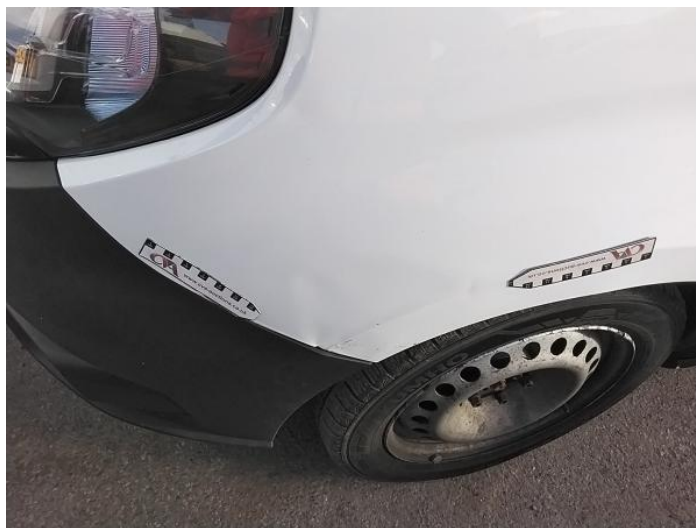
2: Wing nsf Dented With Paint Damage
