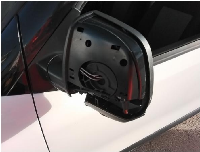
3: Door Mirror Assy nsf Broken Replace
