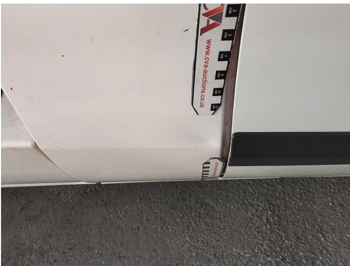
7: B Post os Dented With Paint Damage
