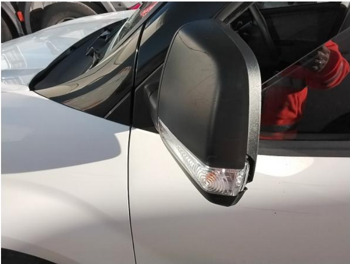
5: Door Mirror Assy nsf Broken Replace
