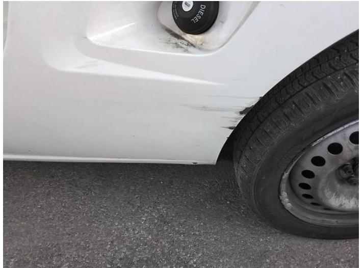
10: Qtr Panel nsr Scratched Over 25mm Thru Paint
