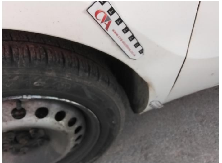
4: Wing nsf Dented With Paint Damage
