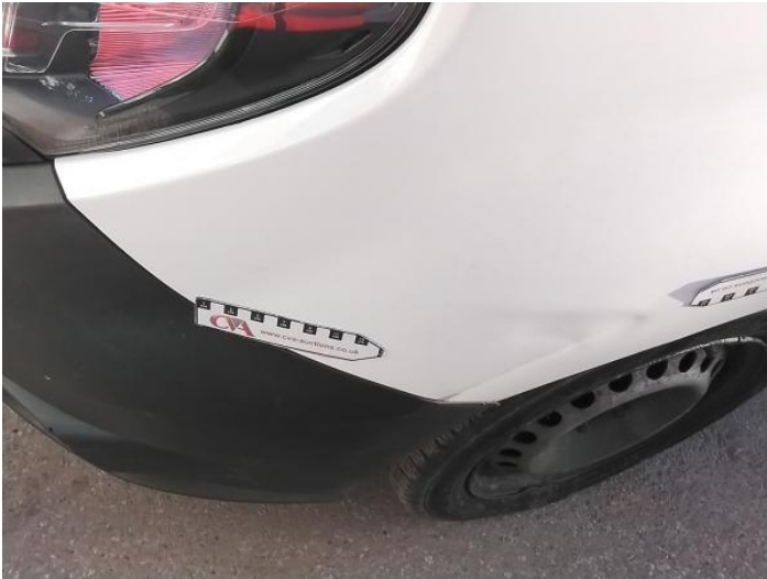
3: Wing nsf Dented With Paint Damage
