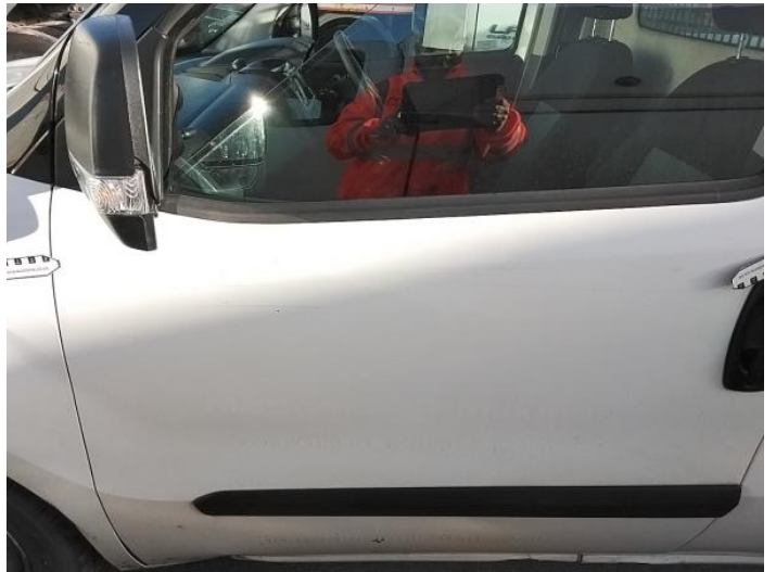
6: Door nsf Scratched Over 25mm Thru Paint
