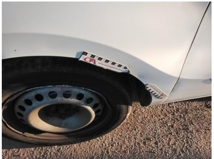
6: Wing nsf Dented Over 30mm
