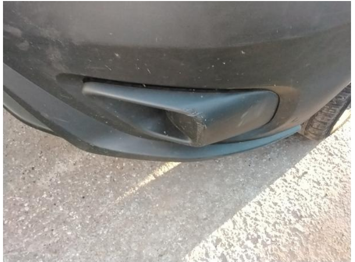
4: Bumper Front Moulding Scuffed (Unpainted) UpTo 100mm
