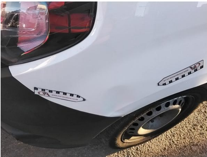
5: Wing nsf Dented Over 30mm
