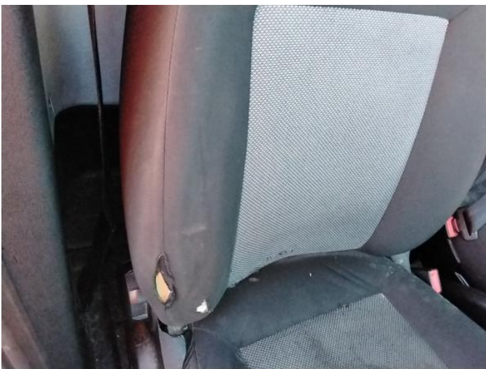
13: Seat Back Cover osf Torn Over 3mm
