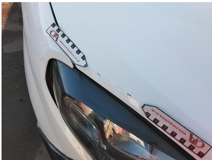
1: Bonnet Dented With Paint Damage
