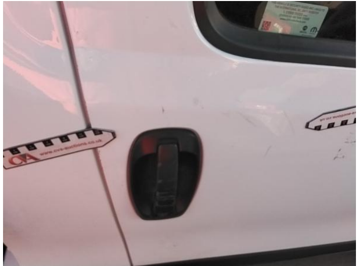
10: Door osf Scratched Over 25mm Thru Paint
