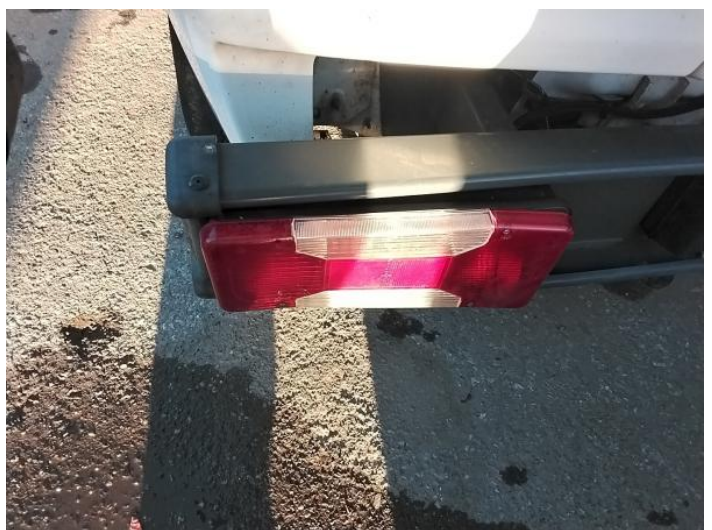
8: Lamp nsr Broken Replace
