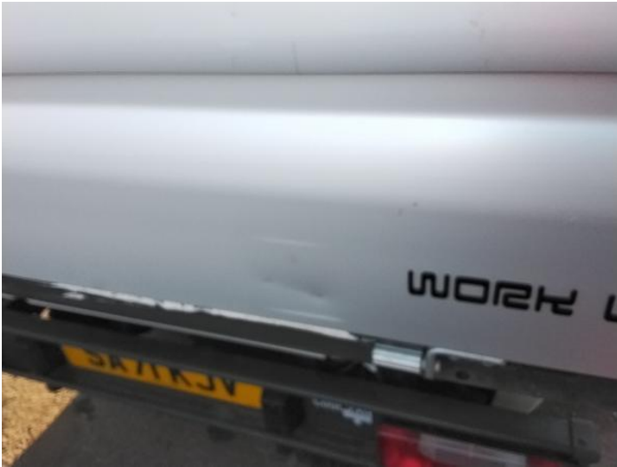
9: Tailgate Dented With Paint Damage
