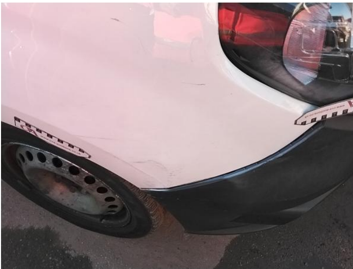
11: Wing osf Dented With Paint Damage
