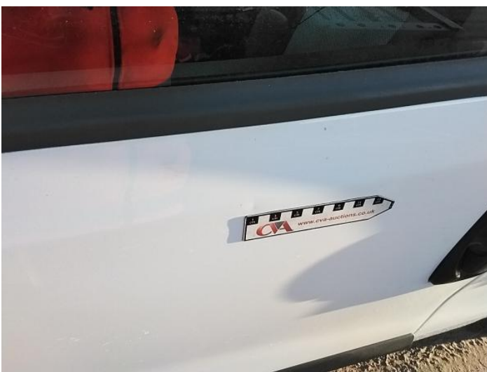
7: Door nsf Dented With Paint Damage
