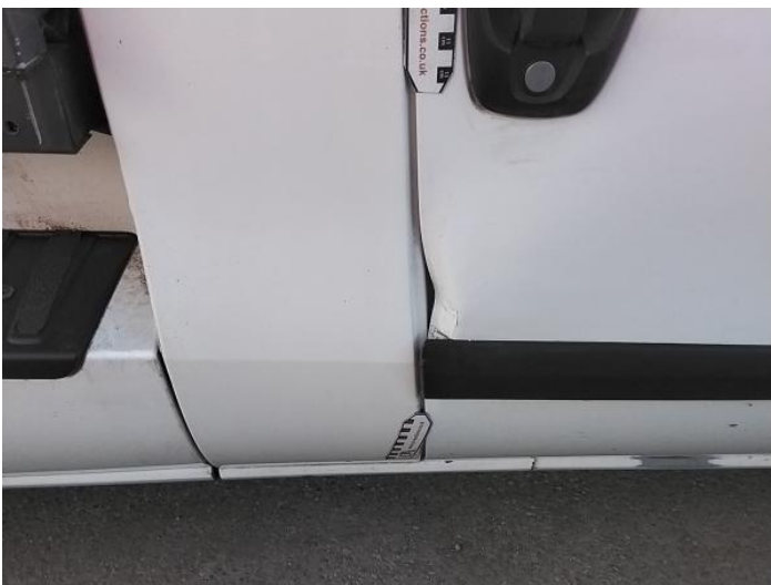
7: Door osf Dented With Paint Damage
