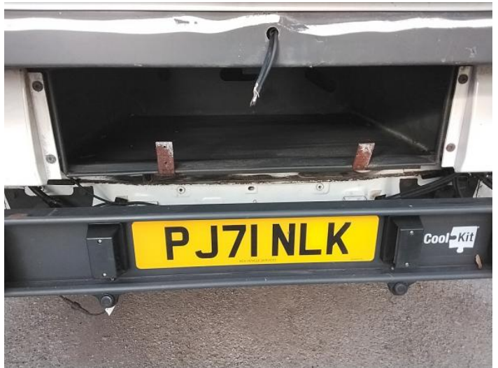
6: Panel Rear Missing Replace
