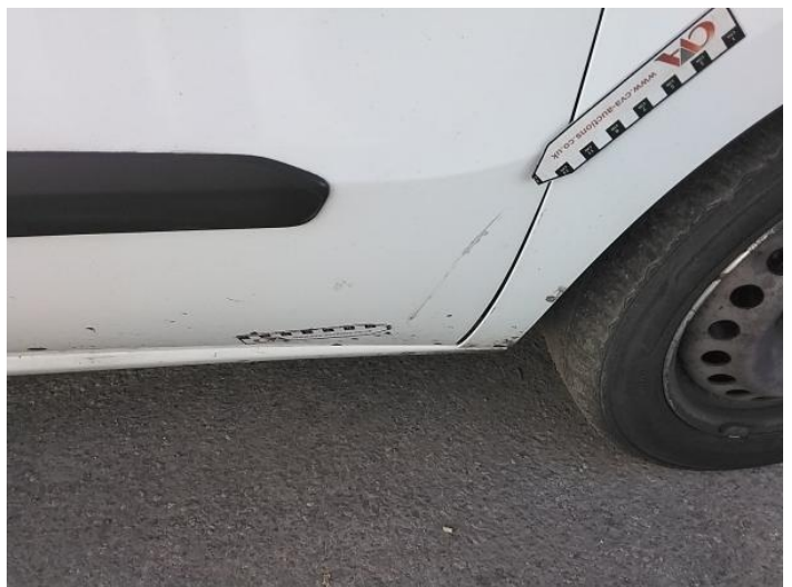
8: Door osf Scratched Over 25mm Thru Paint
