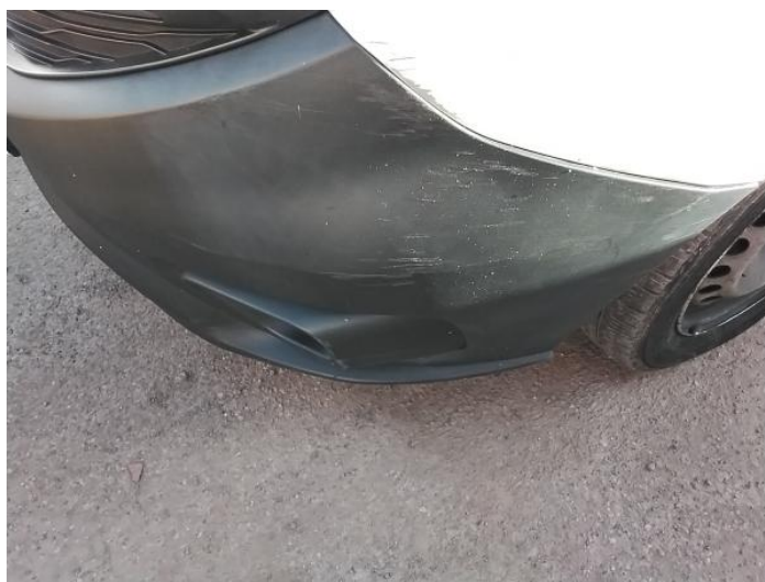
2: Bumper Front Scratched Over 100mm Thru Paint
