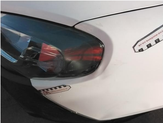
3: Wing nsf Dented With Paint Damage
