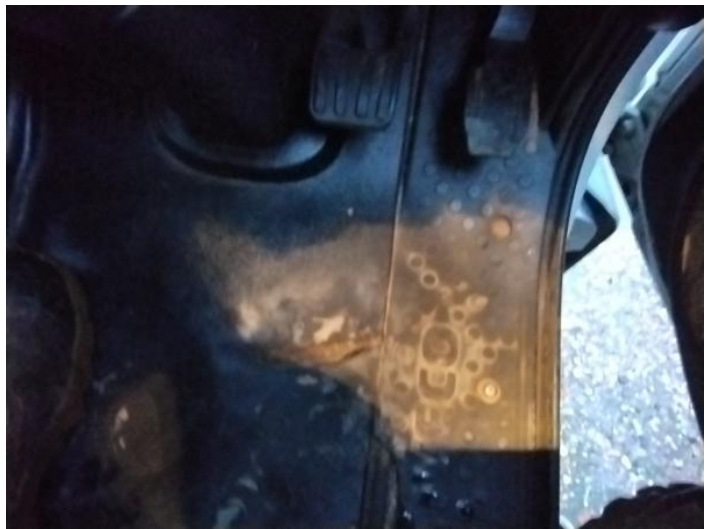
6: Carpets Front Torn Over 10mm
