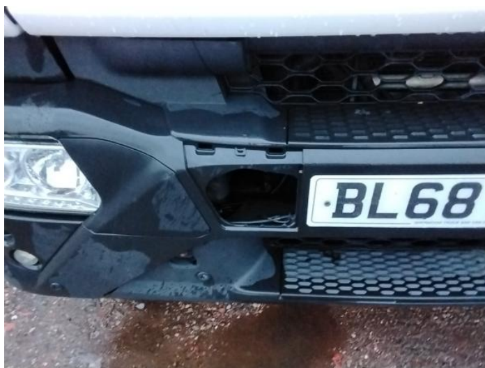
2: Bumper Front Moulding Missing Replace
