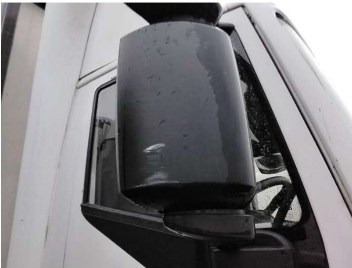
5: Door Mirror Assy osf Scuffed (Unpainted) UpTo 100mm
