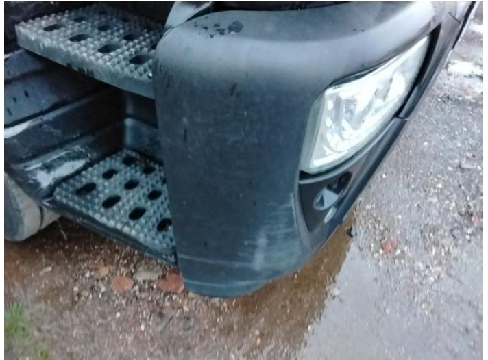
4: Bumper Front Scratched Over 100mm Thru Paint
