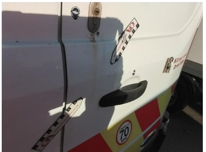
8: Door osr Dented Over 30mm
