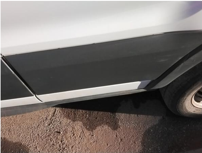
5: Qtr Panel Moulding ns Scuffed (Unpainted) Over 100mm
