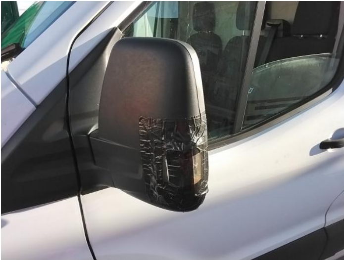
3: Door Mirror Assy nsf Broken Replace
