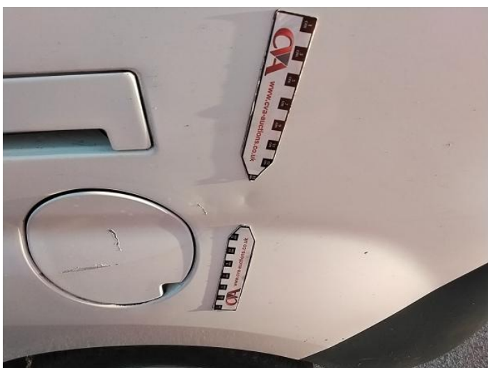
5: Qtr Panel nsr Dented Over 30mm
