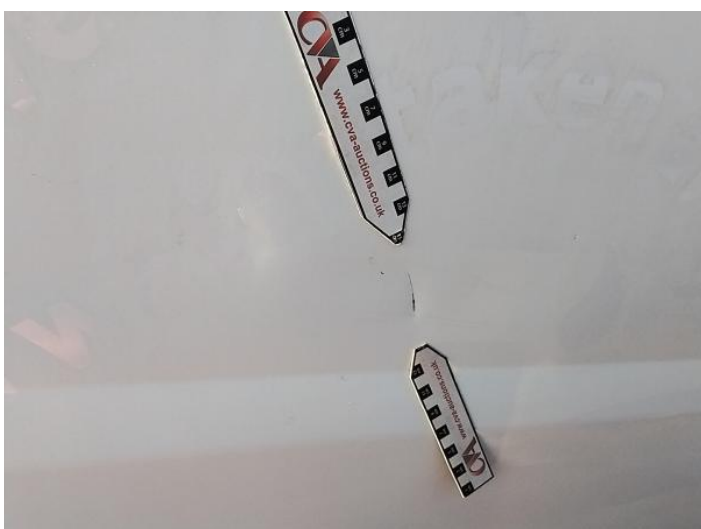
7: Qtr Panel osr Dented With Paint Damage
