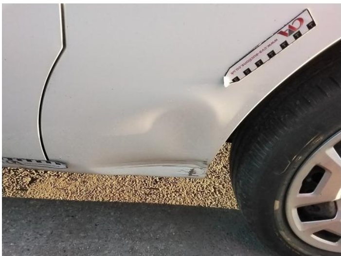
3: Qtr Panel nsr Dented With Paint Damage
