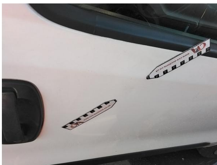
8: Door osf Dented Over 30mm
