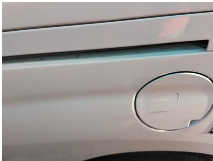
4: Fuel Flap Scratched Over 25mm Thru Paint
