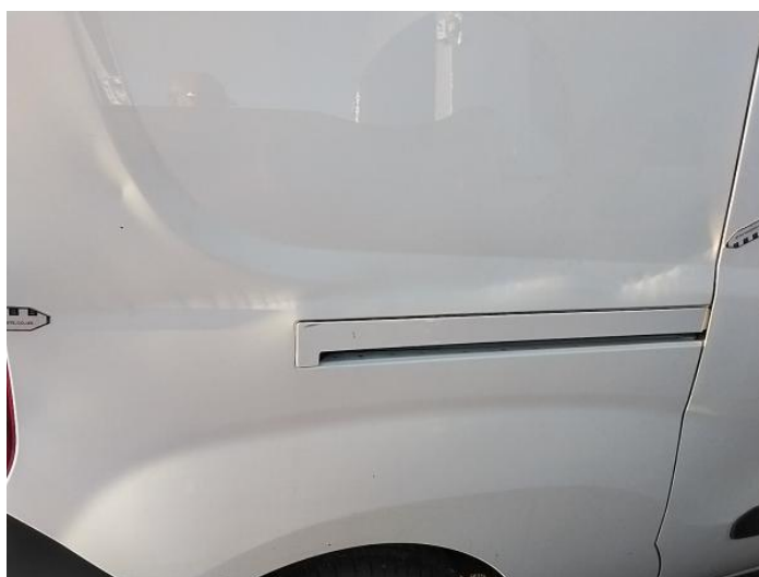
6: Qtr Panel osr Dented Over 30mm
