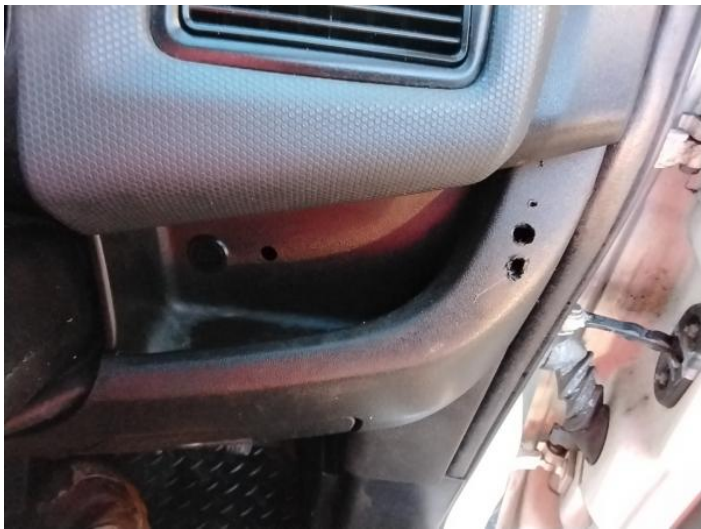
9: Fascia Panel Holed Over 3mm
