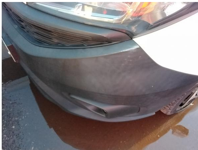
2: Bumper Front Scratched Over 100mm Thru Paint
