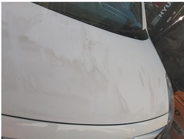
1: Bonnet Scratched Over 25mm Not Thru Paint
