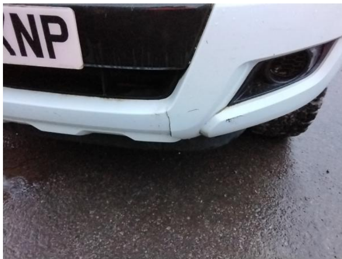
2: Bumper Front Cracked Over 25mm
