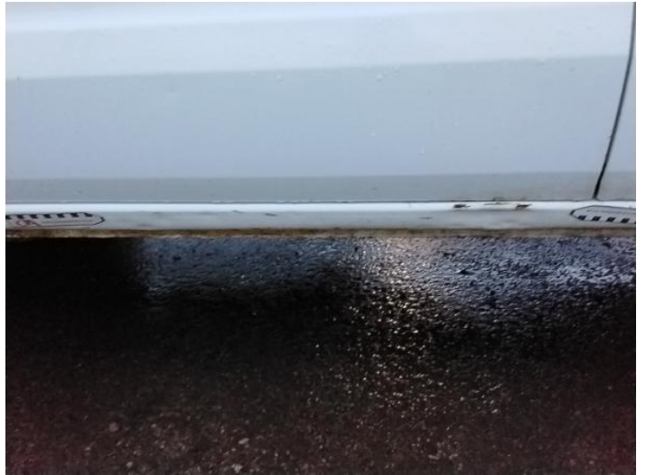
4: Sill ns Dented With Paint Damage
