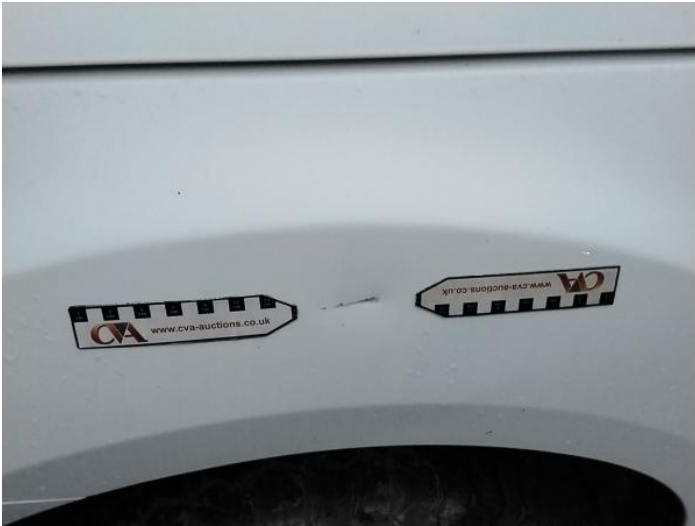
3: Wing nsf Dented With Paint Damage
