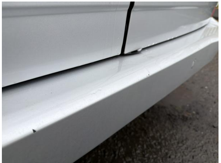
4: Bumper Rear Scratched Over 100mm Thru Paint
