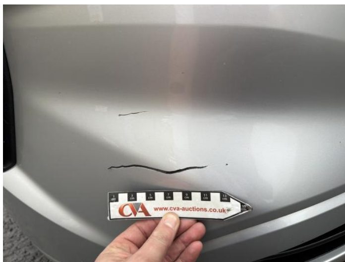
2: Bumper Front Scratched Over 100mm Thru Paint
