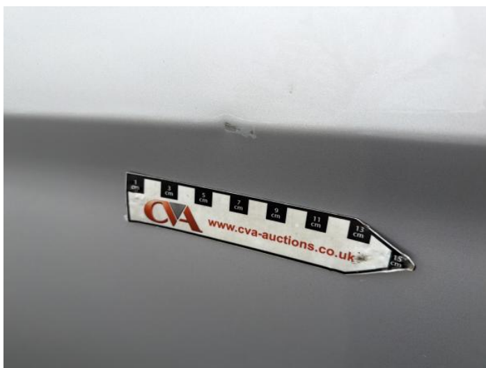
1: Qtr Panel osr Dented With Paint Damage
