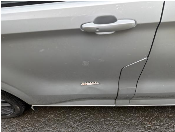
3: Door nsf Dented Over 30mm
