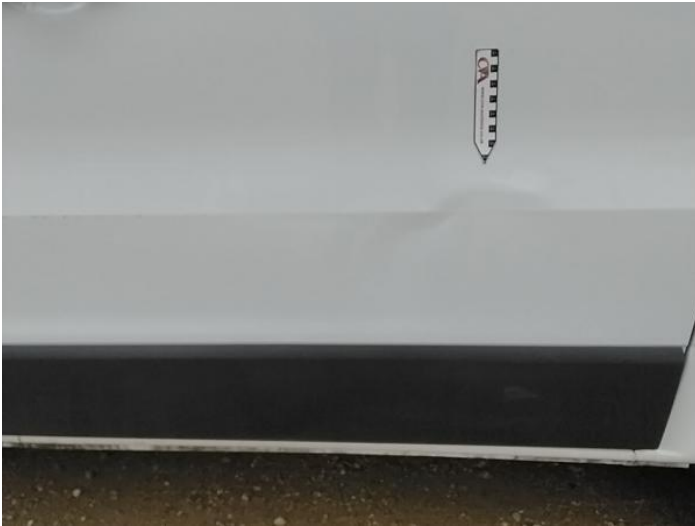
9: Door nsr Dented Between 10mm + 30mm
