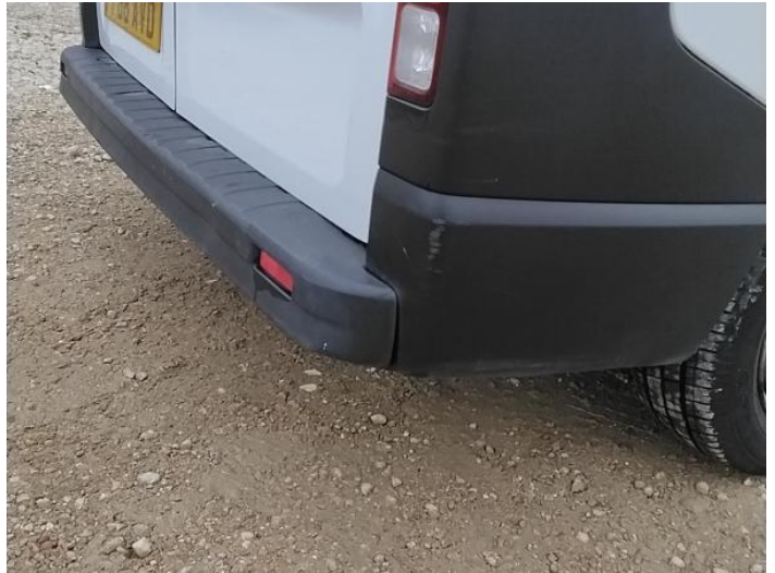
16: Bumper Rear Moulding Scuffed (Unpainted) UpTo 100mm
