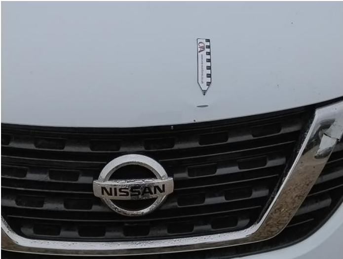
3: Bonnet Dented With Paint Damage
