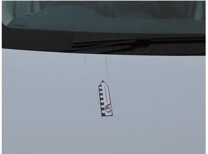
4: Bonnet Scratched Over 25mm Not Thru Paint
