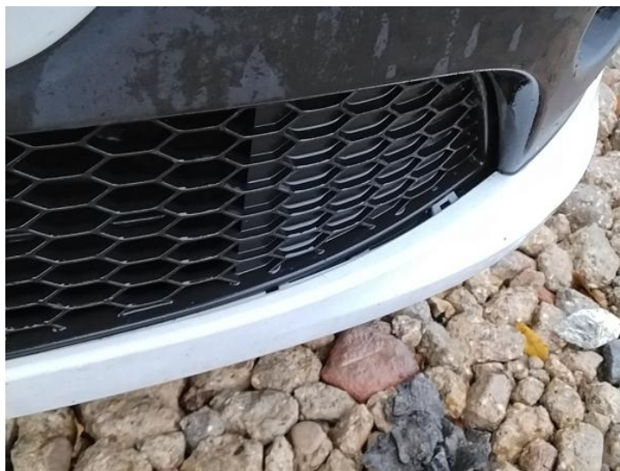
2: Grille Front Broken Replace
