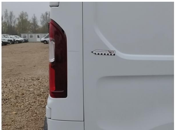
14: Qtr Panel osr Scratched UpTo 25mm Not Thru Paint
