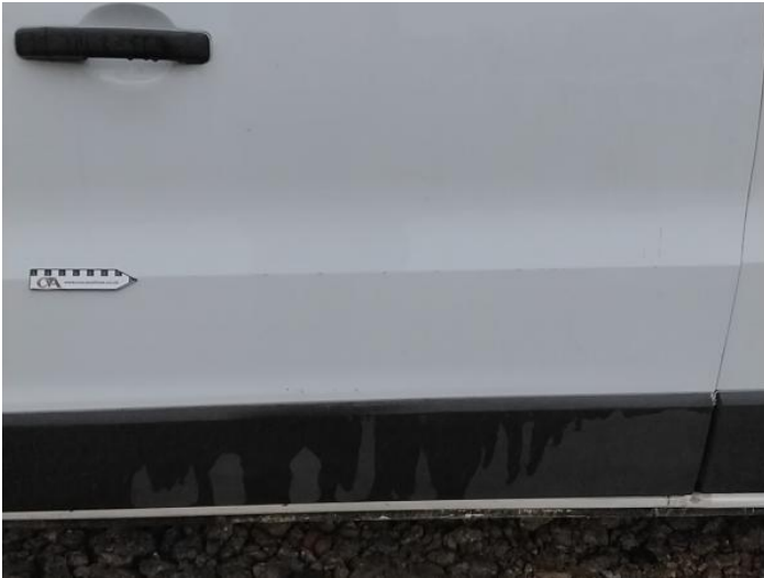
9: Door nsr Scratched Over 25mm Thru Paint
