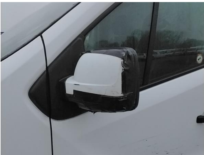
7: Door Mirror Assy nsf Broken Replace
