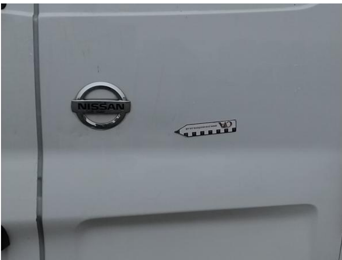
13: Door osr Dented Between 10mm + 30mm
