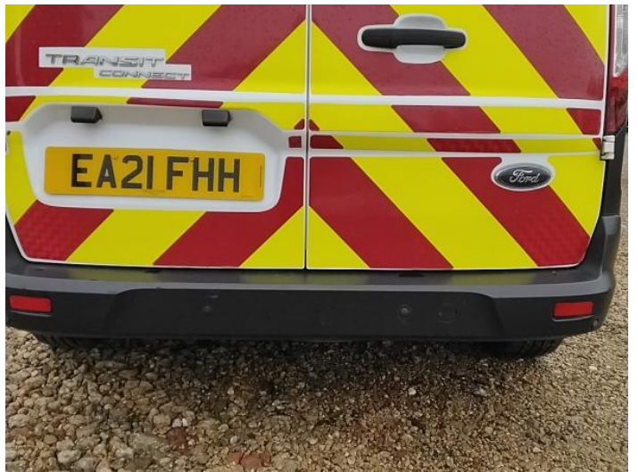
6: Bumper Rear Moulding Scuffed (Unpainted) UpTo 100mm
