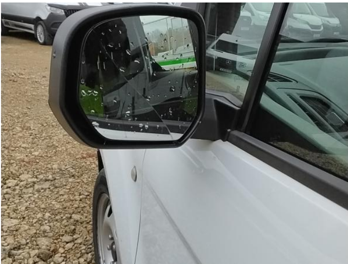
5: Door Mirror Glass ns Broken Replace
