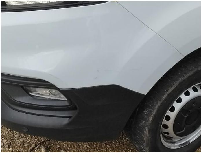
3: Bumper Front Moulding Scuffed (Unpainted) UpTo 100mm
