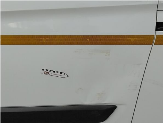
9: Door nsr Dented Over 30mm
