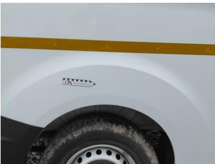
13: Qtr Panel osr Scratched Over 25mm Not Thru Paint
