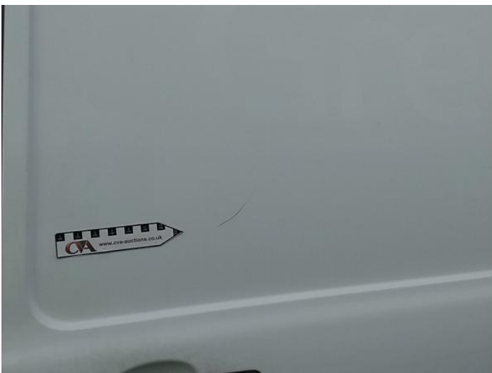
7: Door nsr Scratched UpTo 25mm Not Thru Paint
