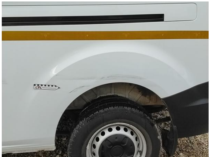
12: Qtr Panel osr Dented With Paint Damage
