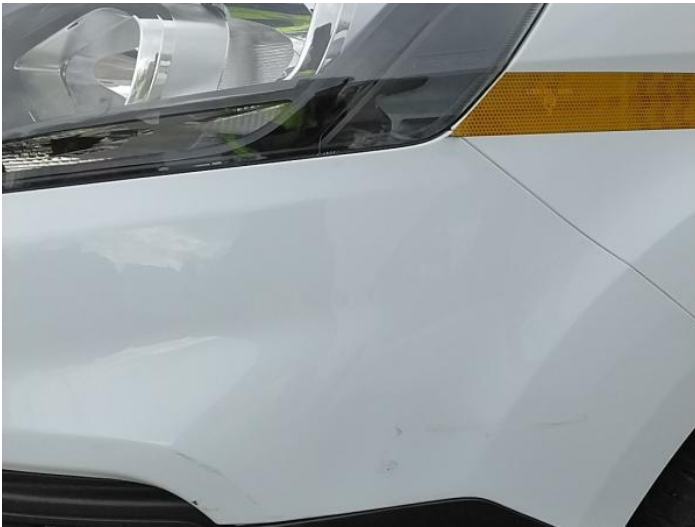
5: Panel Front Scratched Over 25mm Thru Paint
