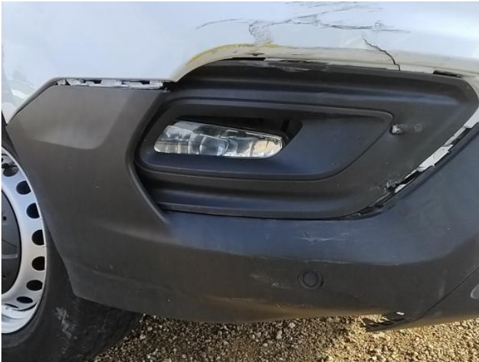
3: Bumper Front Moulding Broken Replace
