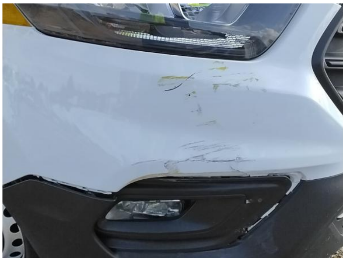
1: Panel Front Cracked Replace
