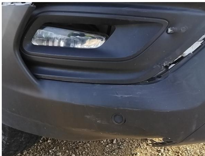
2: Fog Lamp Surround os Broken Replace
