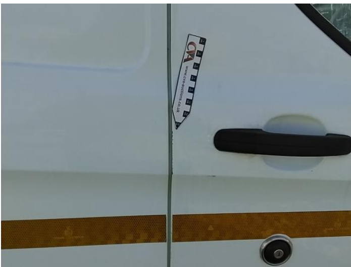
7: Door osf Chipped Edge Chip
