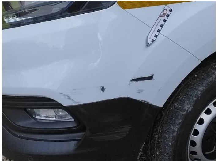
4: Panel Front Scratched Over 25mm Thru Paint
