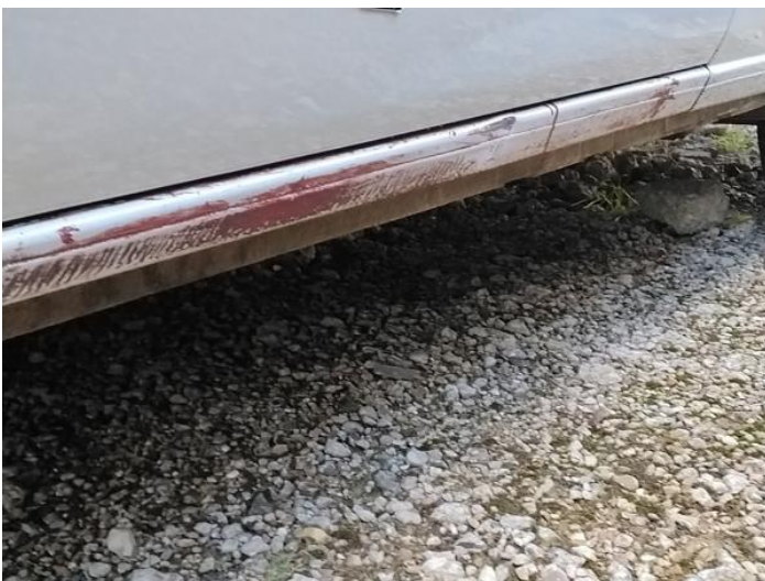
7: Sill ns Dented With Paint Damage
