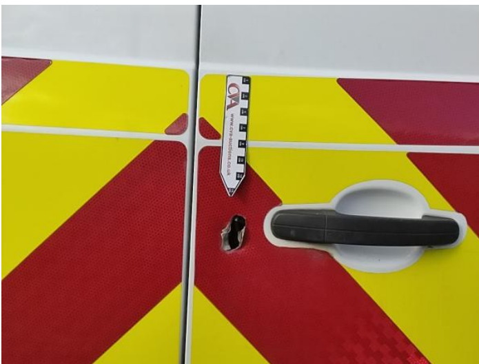
13: Door osr Hole Over 10mm
