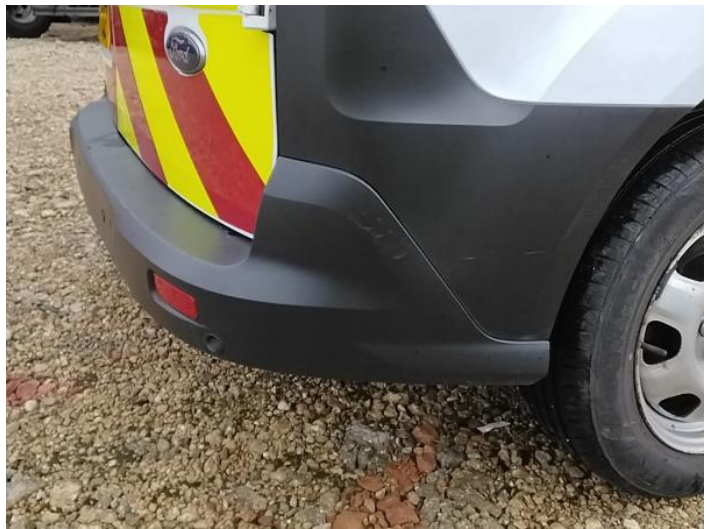
6: Bumper Rear Moulding Scuffed (Unpainted) UpTo 100mm
