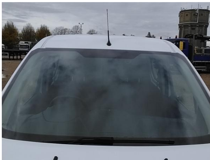
2: Screen Front Chipped UpTo 10mm
