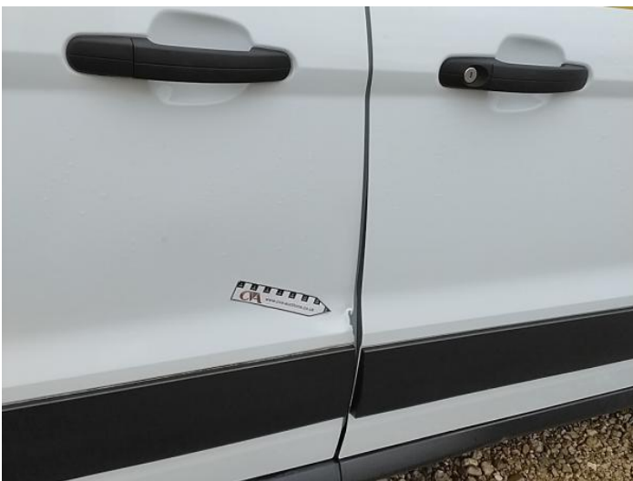
7: Door osr Dented With Paint Damage
