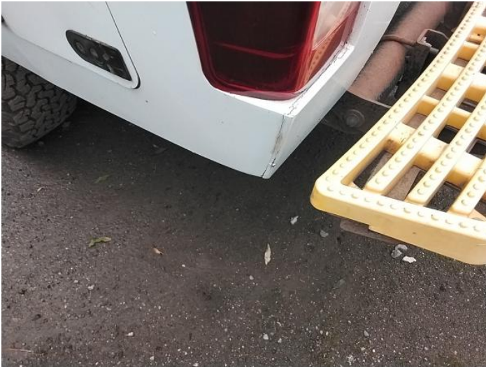
3: Qtr Panel nsr Cracked Replace
