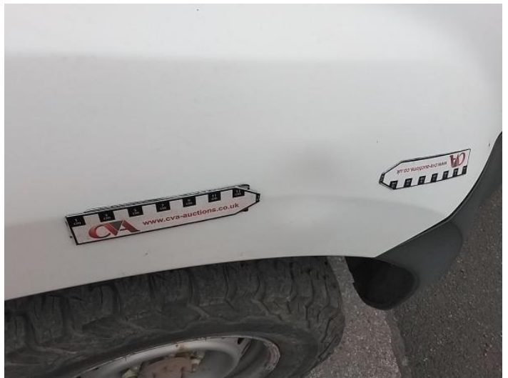
6: Wing osf Dented Over 30mm
