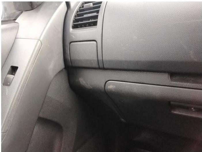
9: Fascia Panel Soiled Heavy
