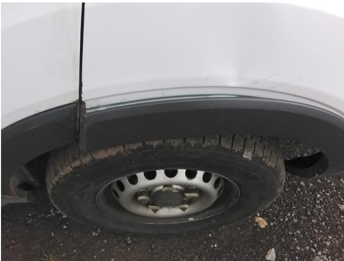
17: Wing Front Arch Extension of Broken Replace
