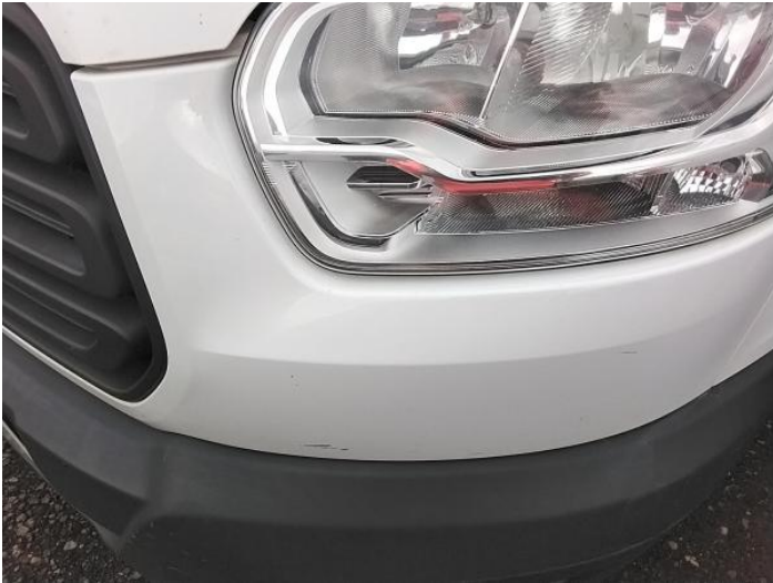
3: Panel Front Scratched Over 25mm Thru Paint
