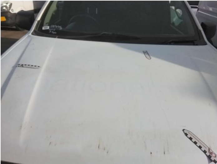
3: Bonnet Scratched Over 25mm Thru Paint
