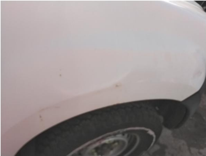
21: Wing osf Dented Over 30% Of Panel
