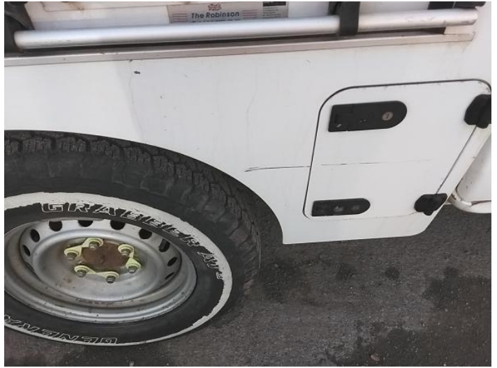
16: Qtr Panel osr Dented With Paint Damage
