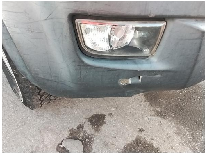
22: Bumper Front Hole Over 25mm
