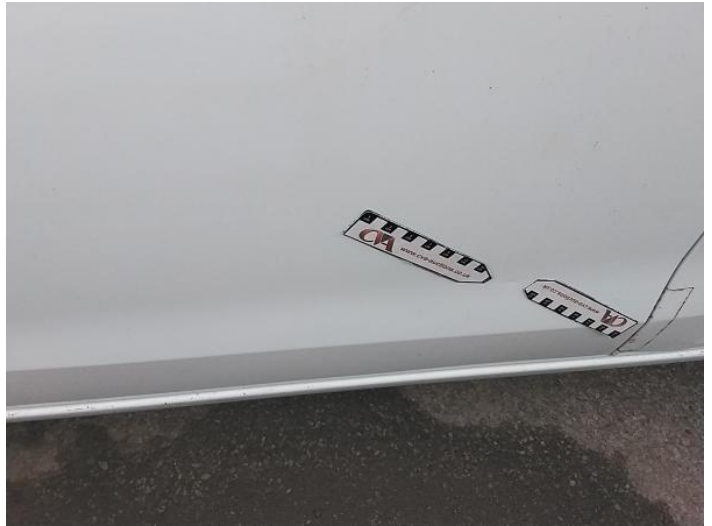
10: Door nsf Dented With Paint Damage
