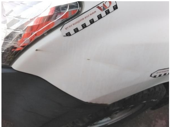
6: Wing nsf Dented With Paint Damage
