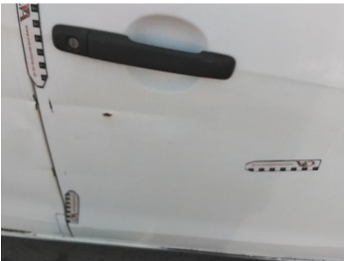
19: Door osf Dented With Paint Damage
