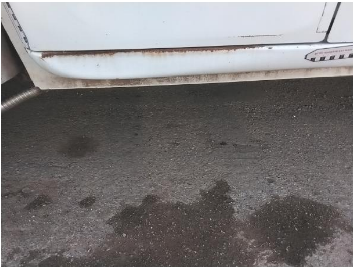
17: Sill os Dented With Paint Damage
