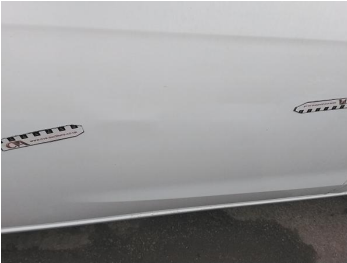
9: Door nsf Dented Over 30mm
