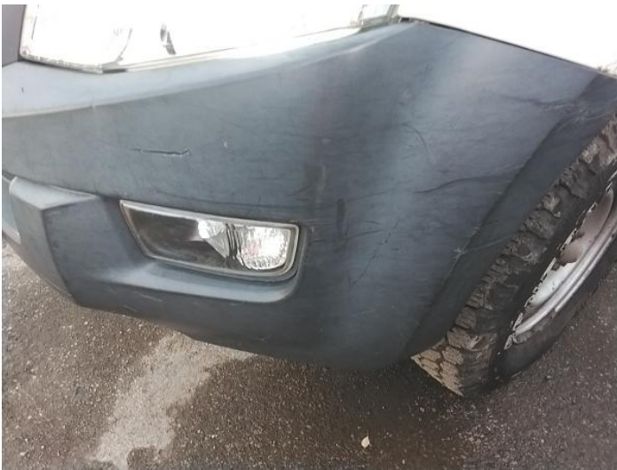
5: Bumper Front Scratched Over 100mm Thru Paint
