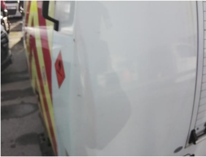
15: Qtr Panel osr Scratched Over 25mm Thru Paint
