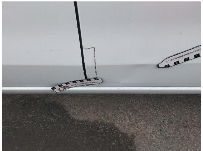
12: Qtr Panel nsr Dented With Paint Damage
