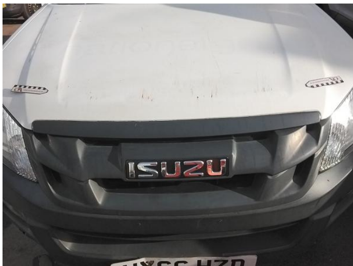
1: Bonnet Dented With Paint Damage
