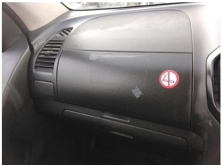
26: Fascia Panel Scuffed Over 25mm
