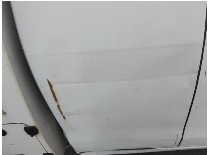
18: Qtr Panel osr Dented Over 30% Of Panel
