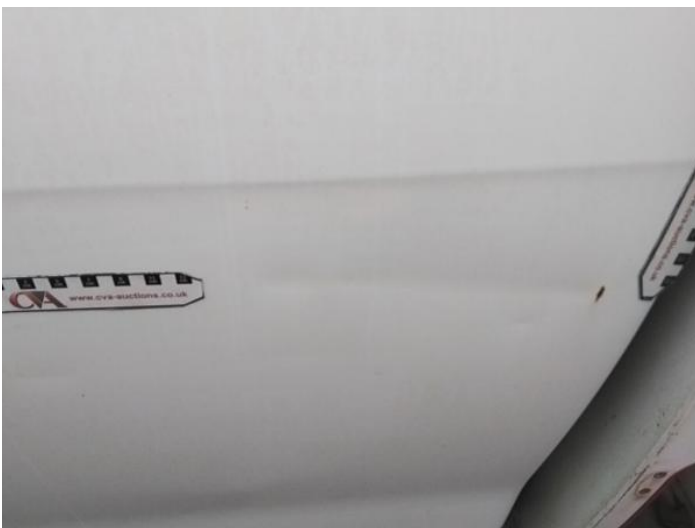
13: Qtr Panel nsr Dented With Paint Damage
