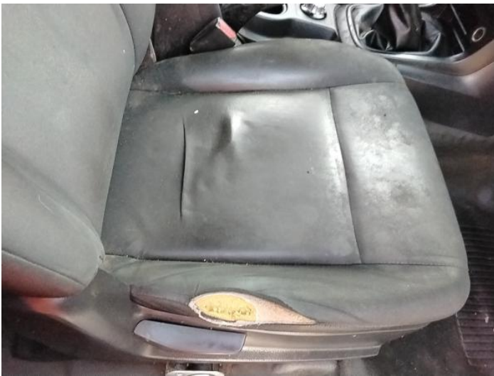
23: Seat Base Cover osf Holed Over 3mm
