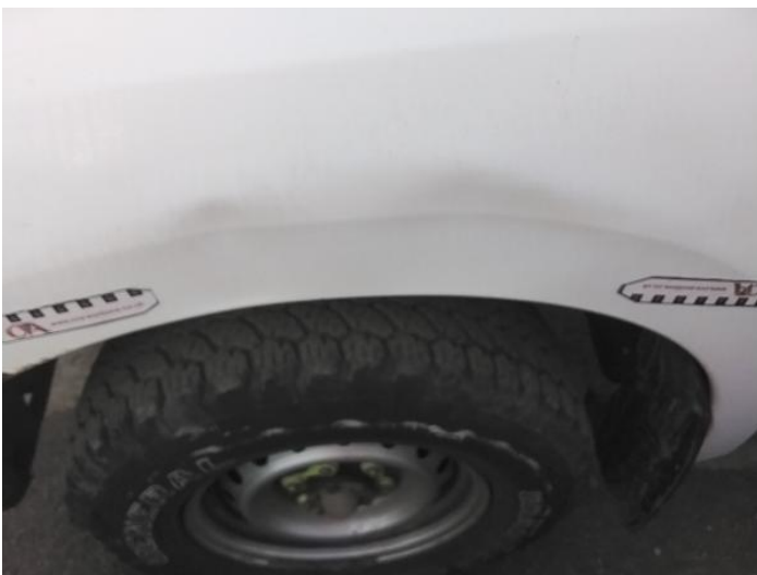
7: Wing nsf Dented Over 30mm
