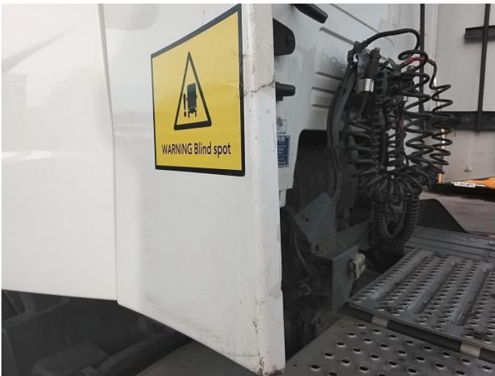
5: Qtr Panel Trim ns Broken Replace
