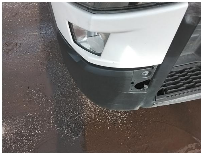
2: Bumper Front Moulding Missing Replace
