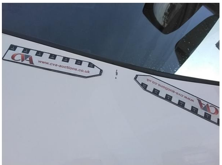
8: Door osf Dented With Paint Damage
