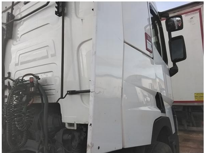
6: Qtr Panel Trim os Broken Replace
