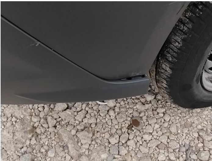
7: Bumper Rear Insecure Action Required
