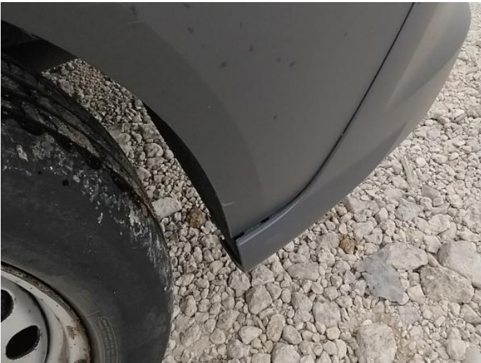
6: Bumper Rear Insecure Action Required
