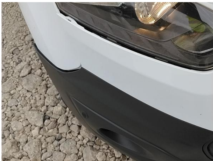
1: Bumper Front Grill Broken Replace
