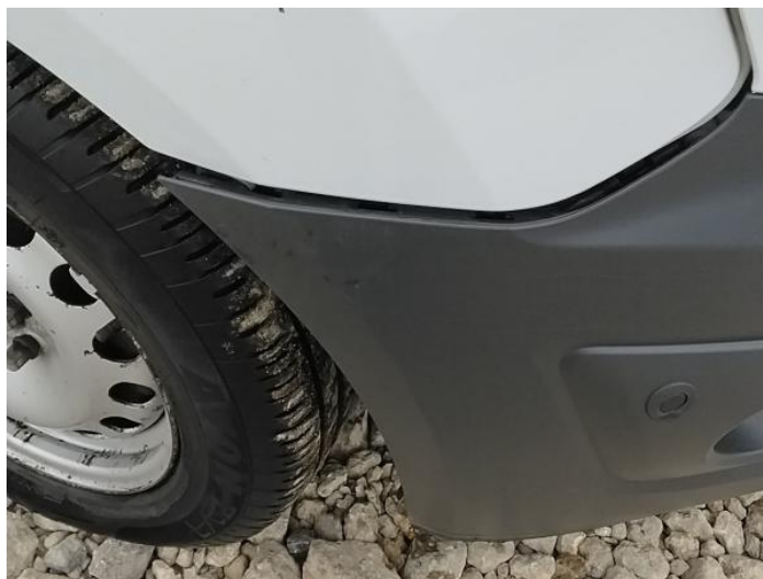
2: Bumper Front Insecure Action Required
