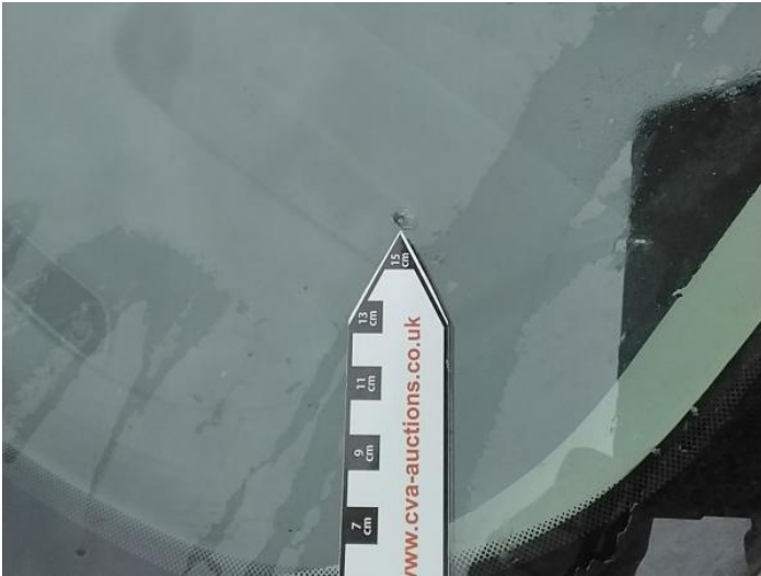
3: Screen Front Chipped UpTo 10mm
