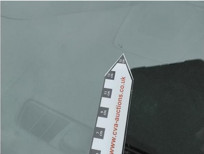
4: Screen Front Chipped UpTo 10mm
