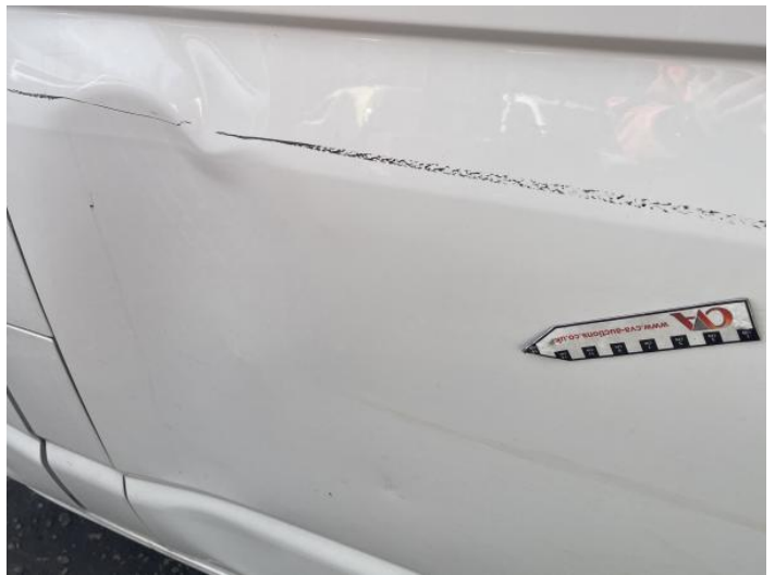
6: Door nsr Dented Over 30% Of Panel
