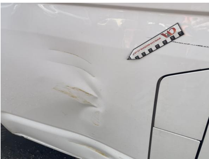
7: Door nsf Dented Over 30% Of Panel
