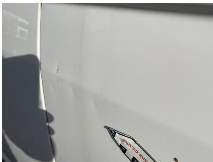
2: Door osf Dented Over 30mm
