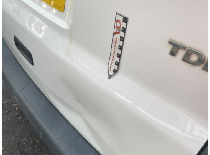
4: Tailgate Dented Over 30% Of Panel
