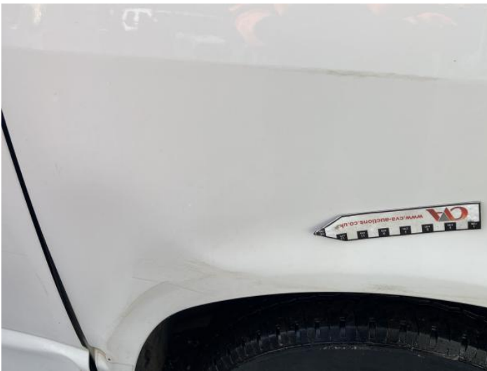
5: Qtr Panel nsr Dented Over 30mm
