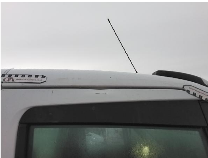
7: Roof Scratched Over 25mm Thru Paint
