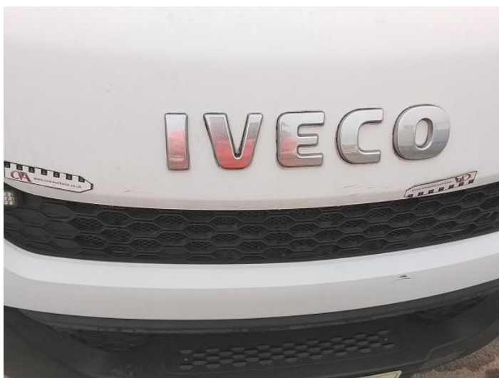
1: Bonnet Scratched Over 25mm Thru Paint
