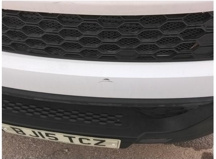
4: Panel Front Scratched Over 25mm Thru Paint
