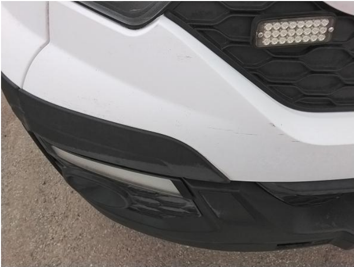
3: Panel Front Scratched Over 25mm Thru Paint
