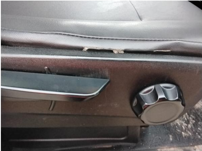
10: Seat Base Cover osf Torn Over 3mm
