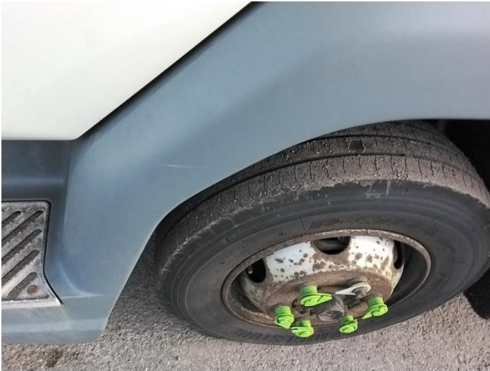
3: Wing nsf Scratched Over 25mm Thru Paint
