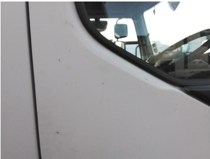
5: Door osf Chipped Multiple Chips
