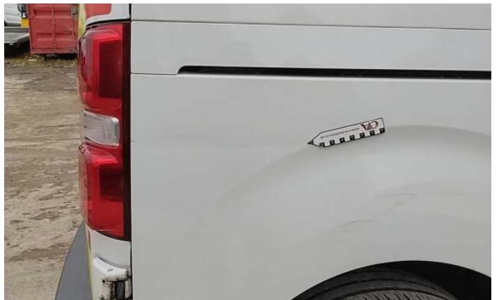
6: Qtr Panel nsr Dented With Paint Damage
