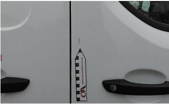
9: Qtr Panel osr Dented With Paint Damage
