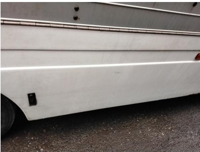
7: Qtr Panel Moulding os Scratched (Painted) Over 25mm Thru Paint
