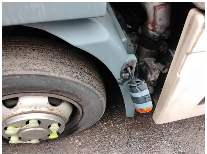
8: Flasher Side Repeater ns Broken Replace
