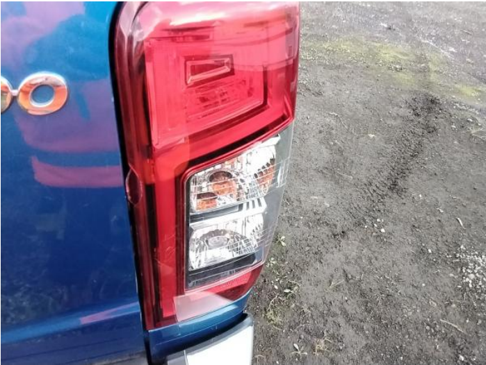
10: Lamp osr Broken Replace
