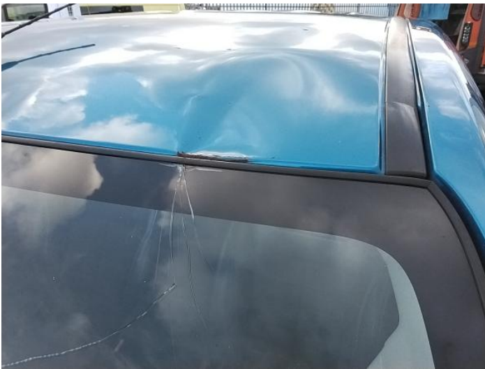
5: Roof Dented With Paint Damage
