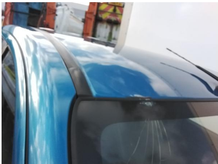
1: Roof Dented With Paint Damage
