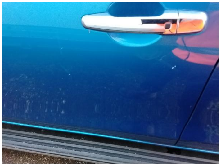
6: Door nsf Chipped Multiple Chips
