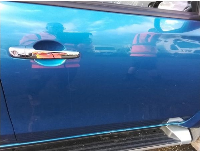
14: Door osf Chipped Multiple Chips
