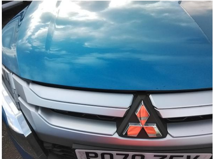
4: Bonnet Poor Previous Repair Poor Colour
