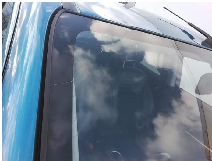
2: Screen Front Cracked Replace
