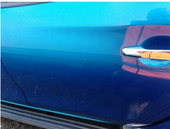
7: Door nsr Chipped Multiple Chips
