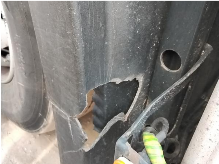
4: Moulding osf Wing Broken Replace
