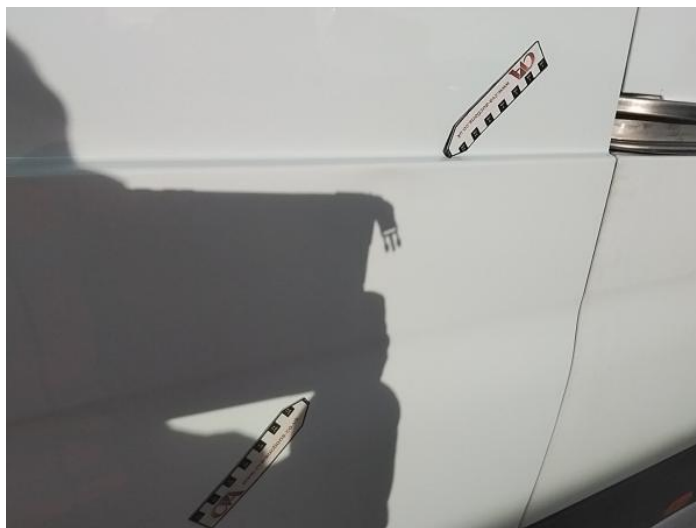
2: Qtr Panel nsr Dented Over 30mm
