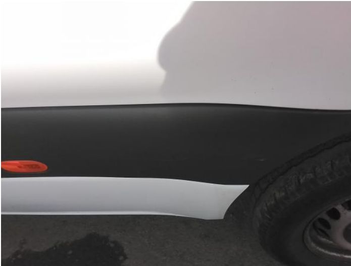
3: Qtr Panel Moulding ns Scuffed (Unpainted) Over 100mm
