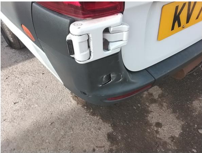
5: Bumper Rear Moulding Broken Replace
