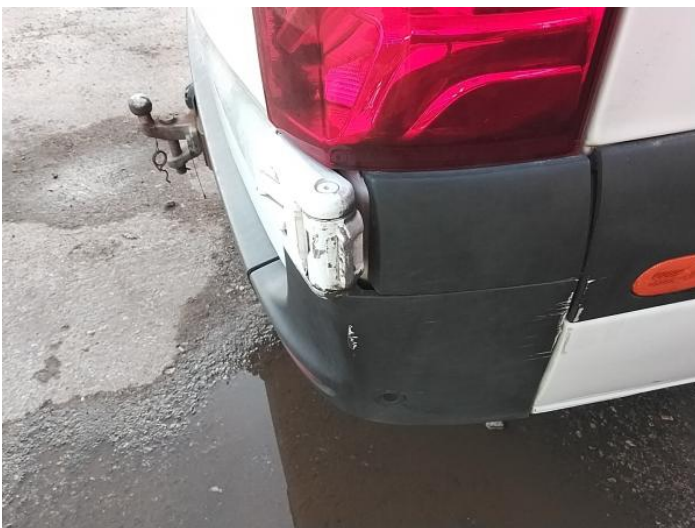
7: Bumper Rear Moulding Scuffed (Unpainted) Over 100mm
