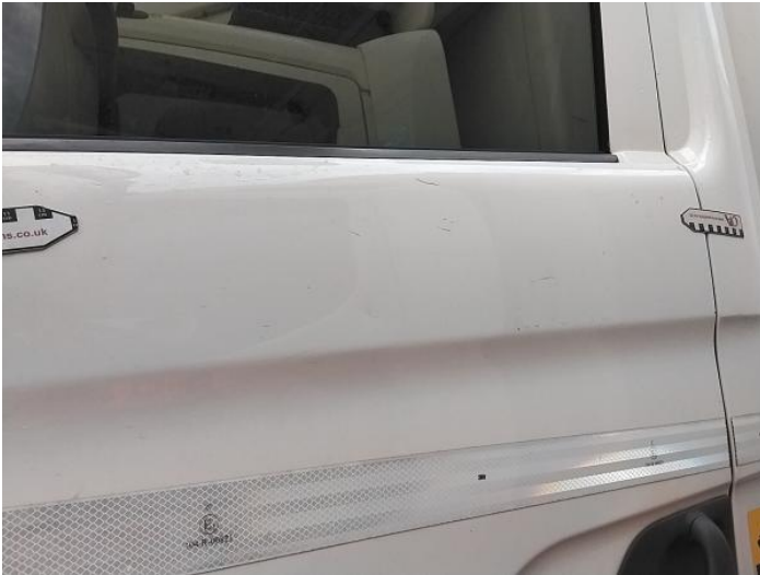
3: Door nsf Scratched Over 25mm Thru Paint
