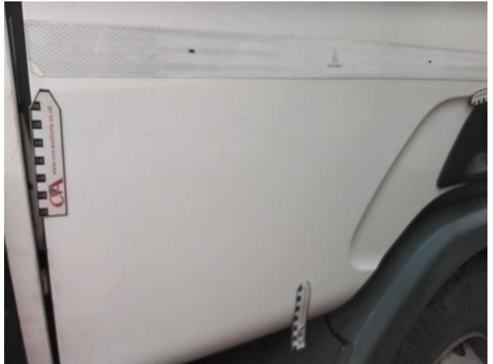
4: Door nsf Scratched Over 25mm Thru Paint
