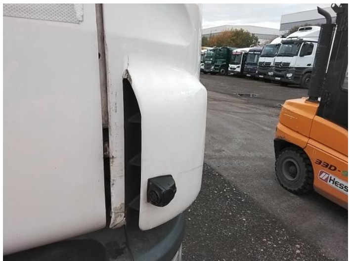
8: Panel Front Cracked Replace
