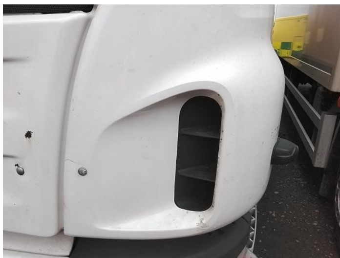
2: Panel Front Cracked Replace
