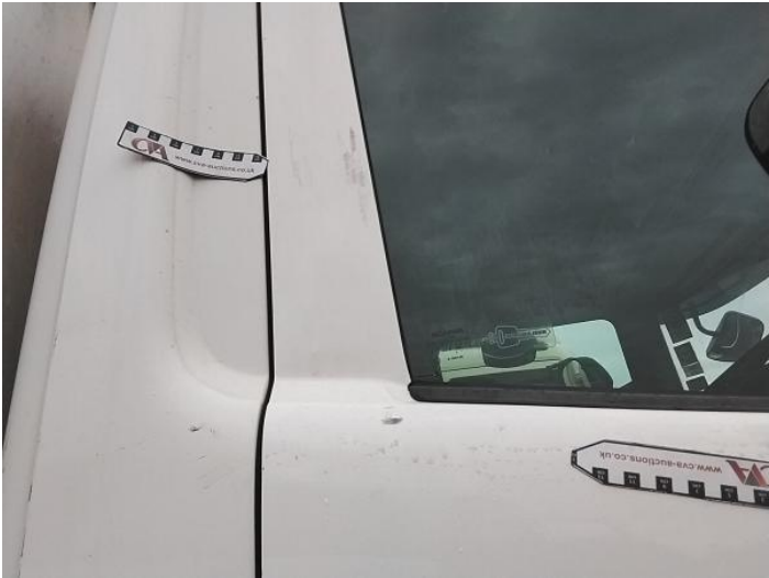
9: Door osf Scratched Over 25mm Thru Paint
