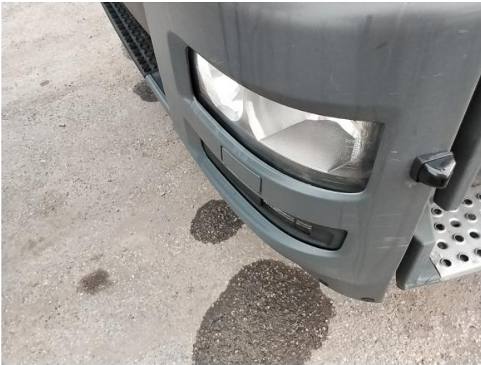
5: Bumper Front Moulding Scuffed (Unpainted) Over 100mm
