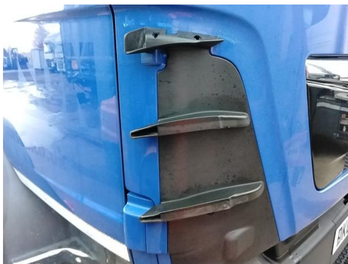
2: Panel Front Missing Replace
