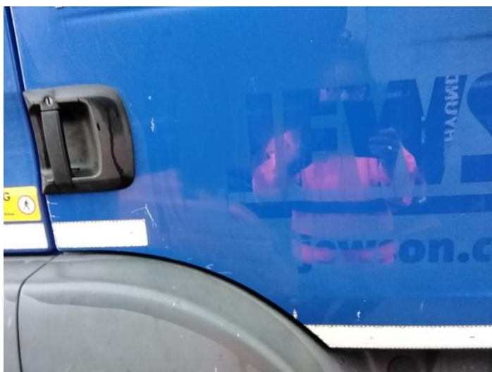
1: Door osf Scratched Over 25mm Thru Paint
