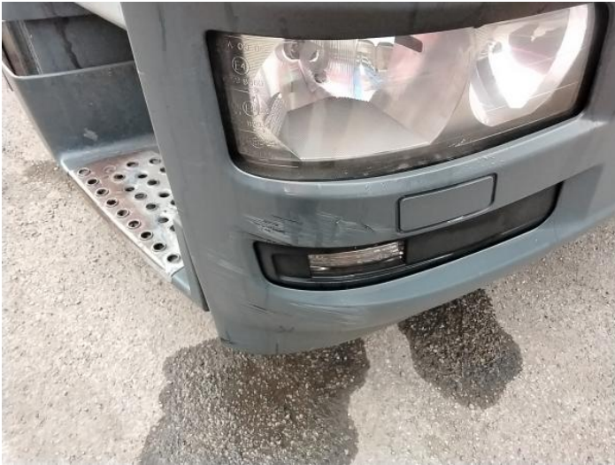
3: Bumper Front Moulding Scuffed (Unpainted) Over 100mm
