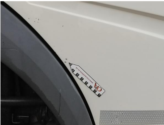
11: Door osf Scratched UpTo 25mm Thru Paint
