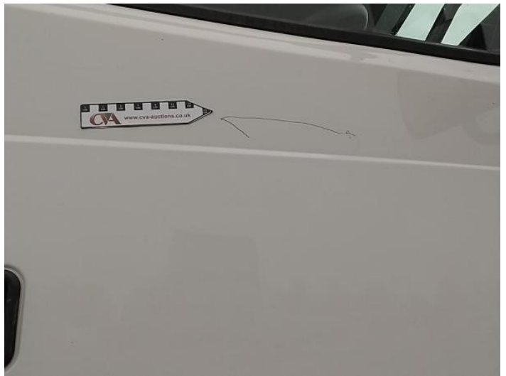
12: Door osf Scratched UpTo 25mm Thru Paint
