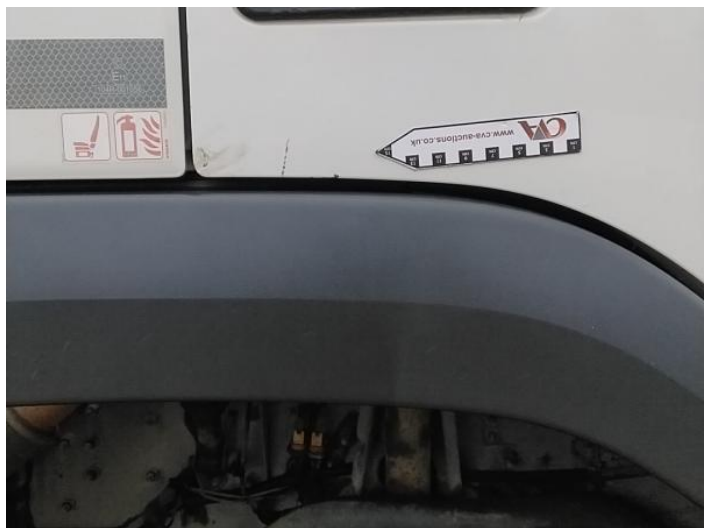
8: Door osf Scratched UpTo 25mm Thru Paint
