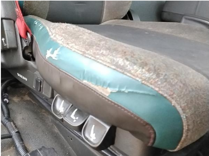
10: Seat Base Cover osf Torn Over 3mm
