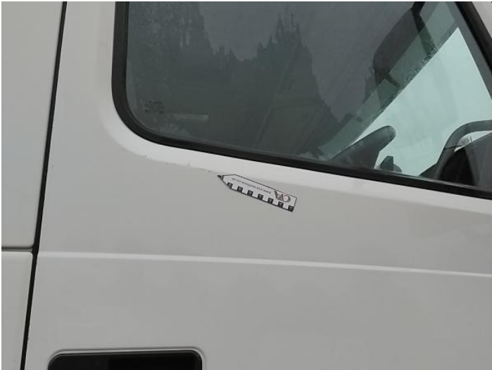
9: Door osf Scratched UpTo 25mm Thru Paint
