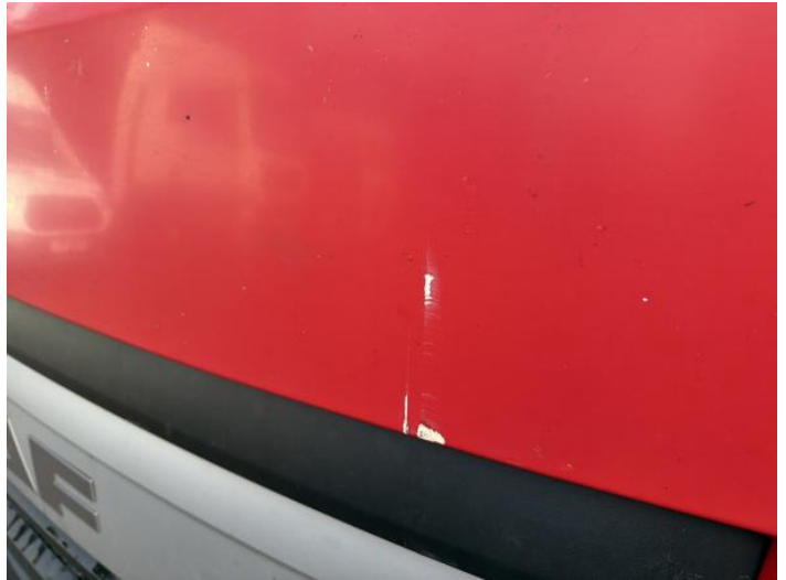
4: Bonnet Dented With Paint Damage
