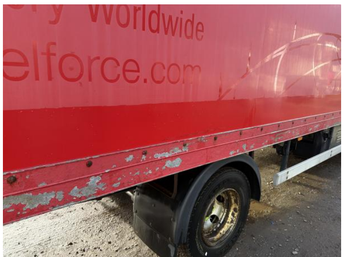
8: Qtr Panel osr Chipped Multiple Chips
