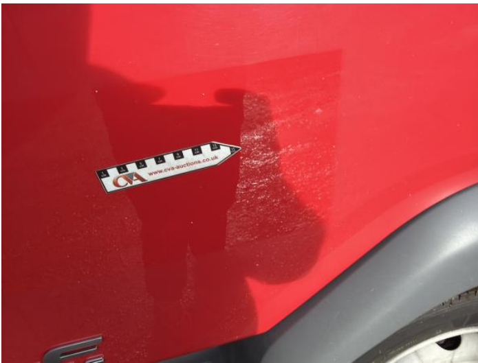
5: Door nsf Chipped Multiple Chips
