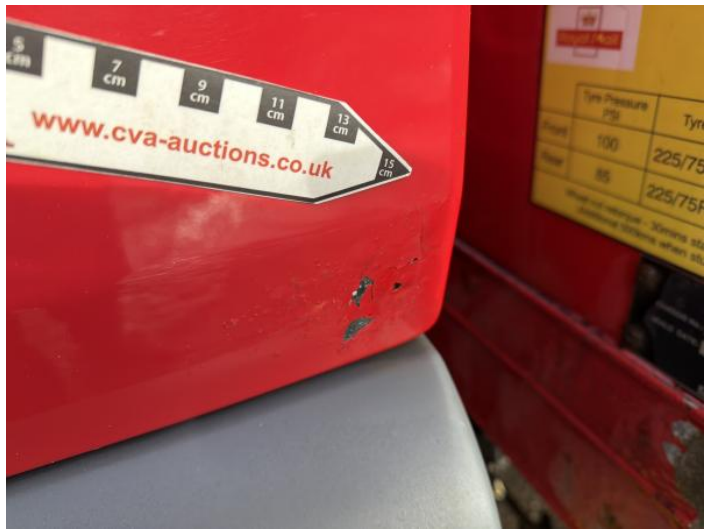
6: B Post ns Rusted Over 5mm
