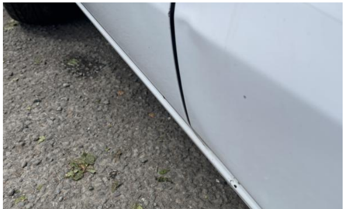
6: Qtr Panel nsr Dented With Paint Damage
