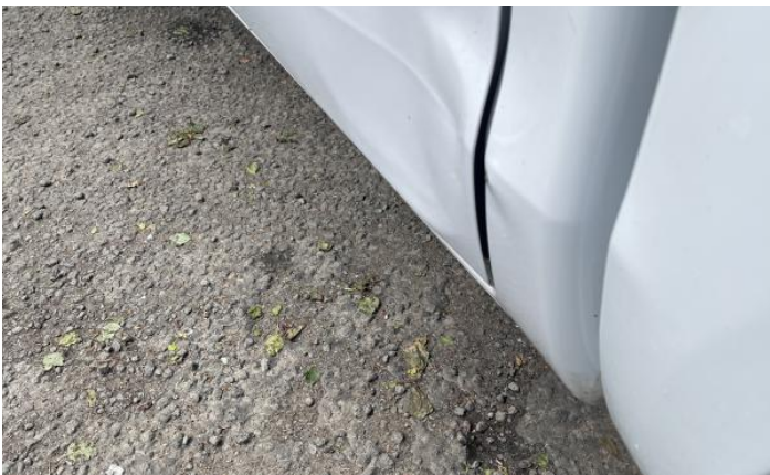
5: Tailgate Dented With Paint Damage
