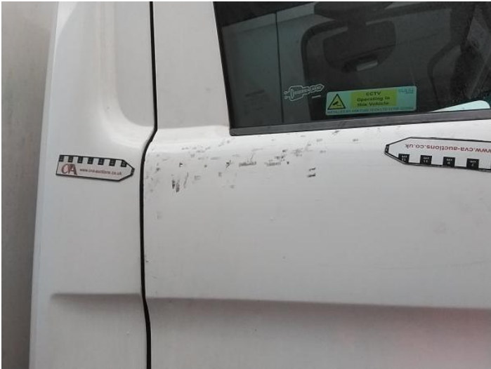
9: Door osf Dented With Paint Damage
