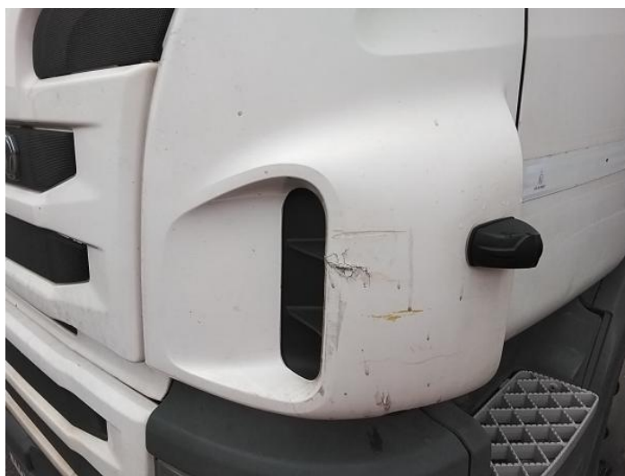
2: Panel Front Cracked Replace
