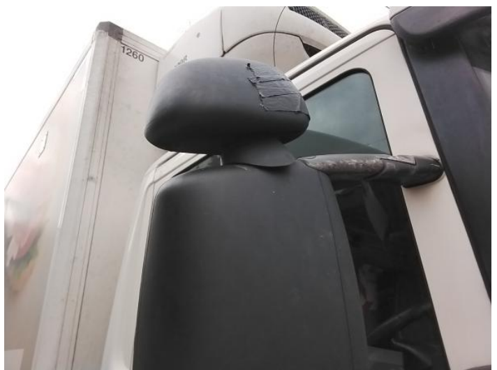
8: Door Mirror Assy osf Broken Replace
