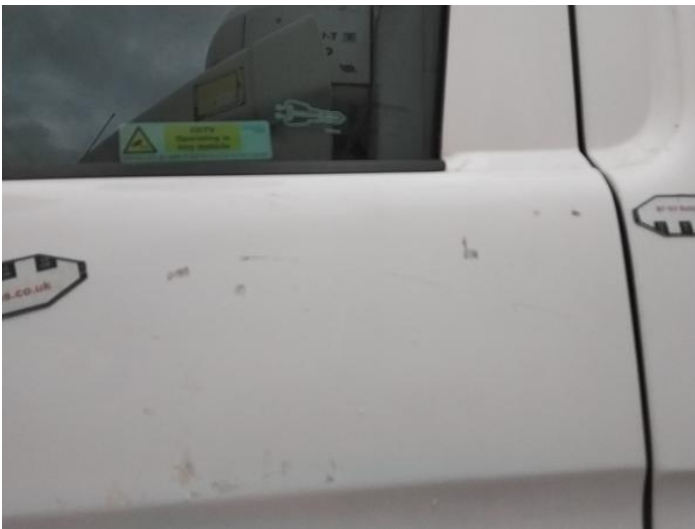
5: Door nsf Scratched Over 25mm Thru Paint
