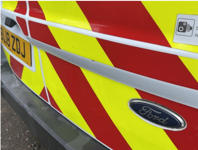
5: Tailgate Dented With Paint Damage
