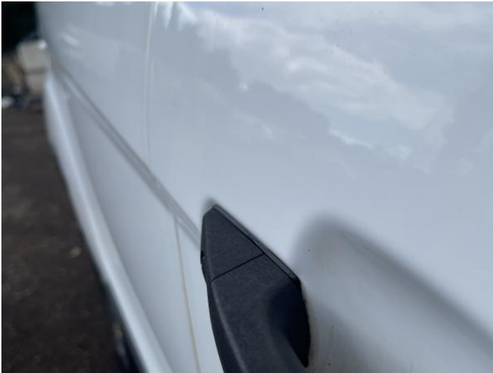
3: Door osf Dented Between 10mm + 30mm
