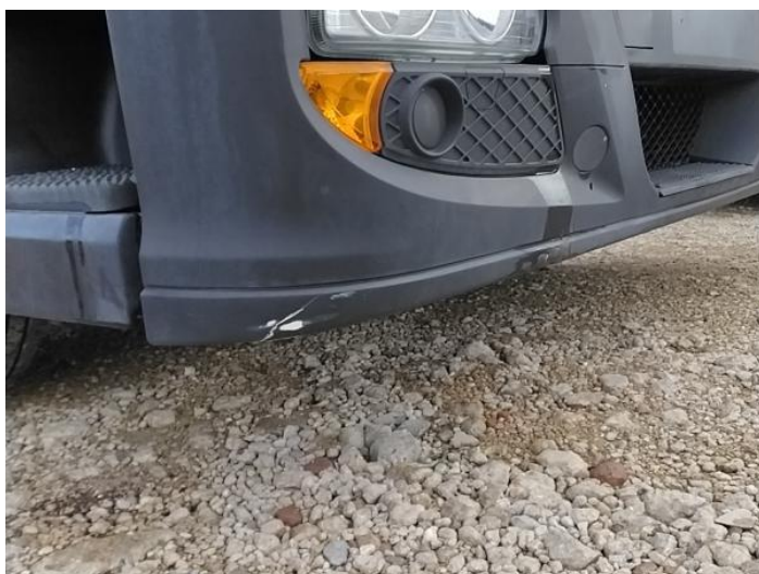
1: Bumper Front Moulding Scuffed (Unpainted) UpTo 100mm
