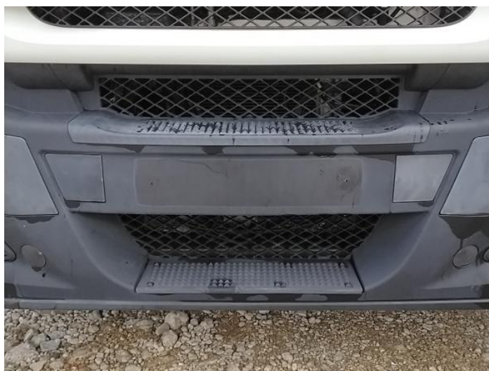
2: Number Plate Front Missing Replace
