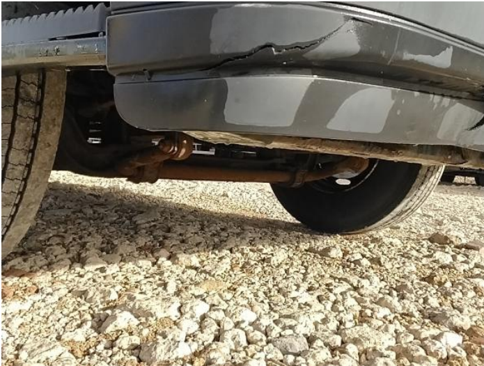
3: Bumper Front Moulding Broken Replace
