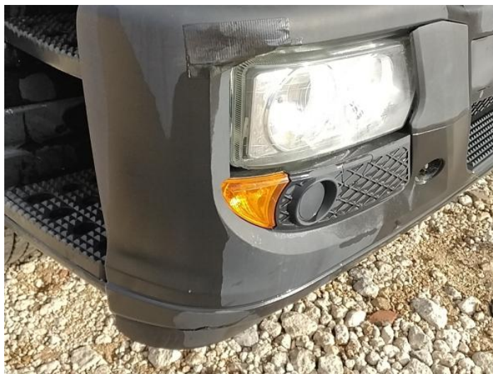
2: Fog Lamp Surround os Broken Replace
