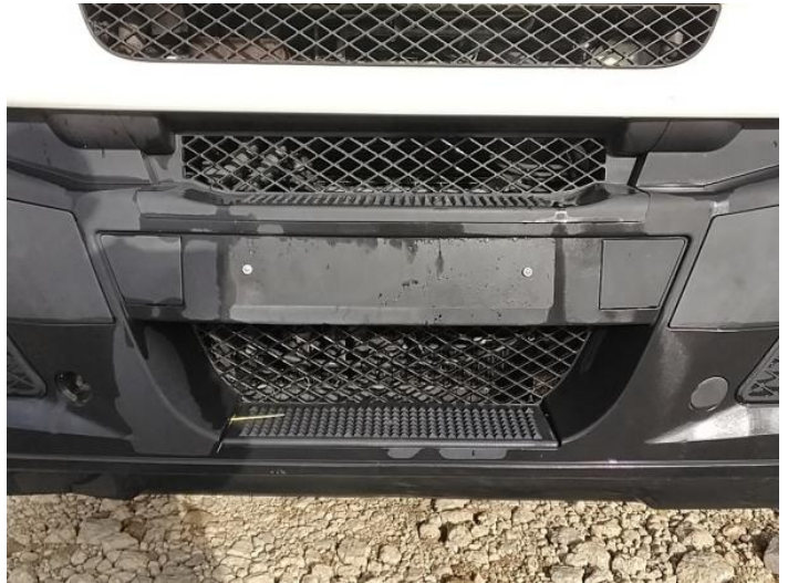
6: Number Plate Front Missing Replace
