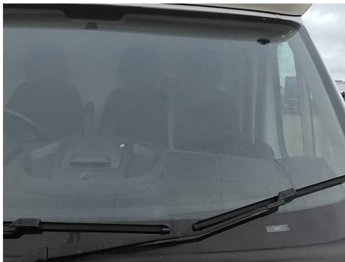
2: Screen Front Chipped Over 10mm
