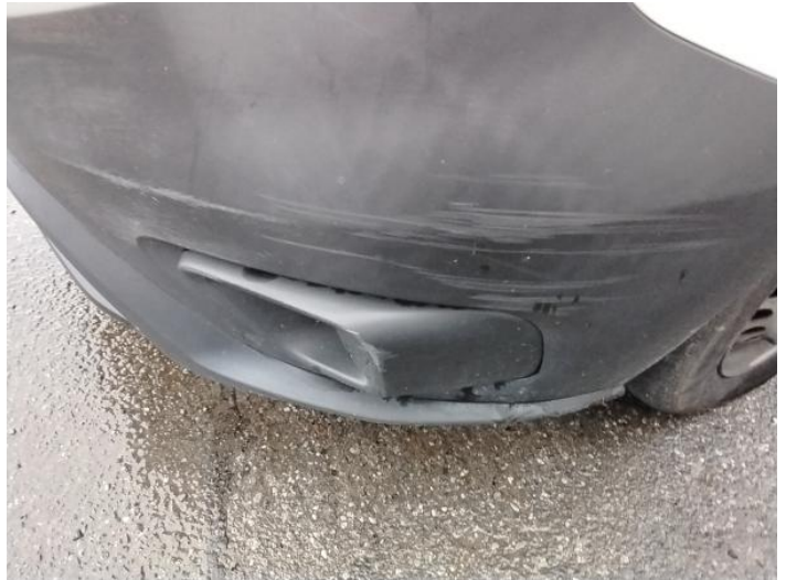
4: Bumper Front Scratched Over 100mm Thru Paint
