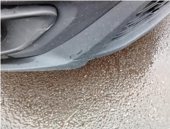
3: Bumper Front Cracked Over 25mm
