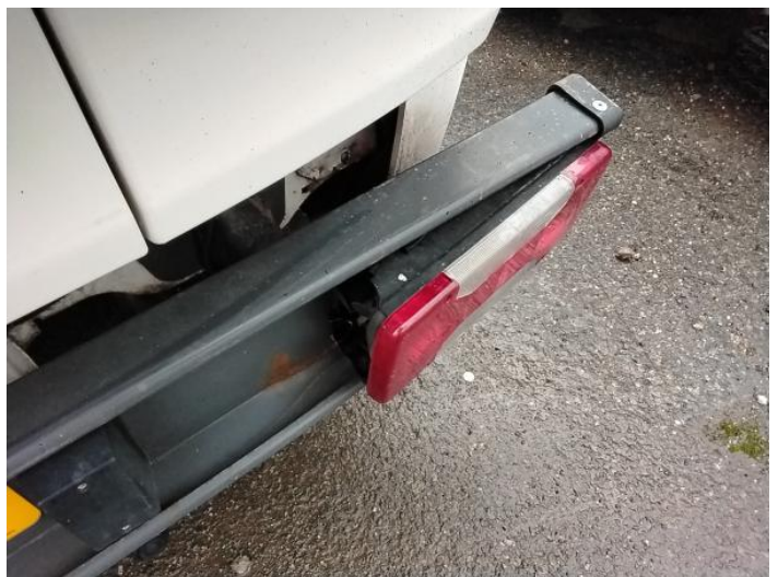
8: Lamp osr Broken Replace
