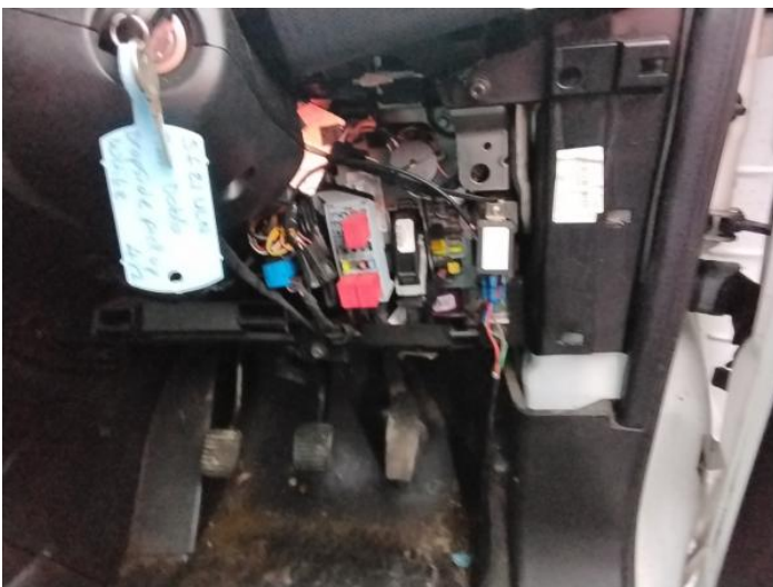
19: Fascia Panel Missing Replace
