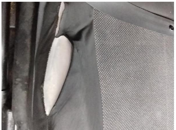
20: Seat Base Cover osf Torn Over 3mm
