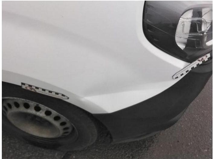
16: Wing osf Dented Over 30mm
