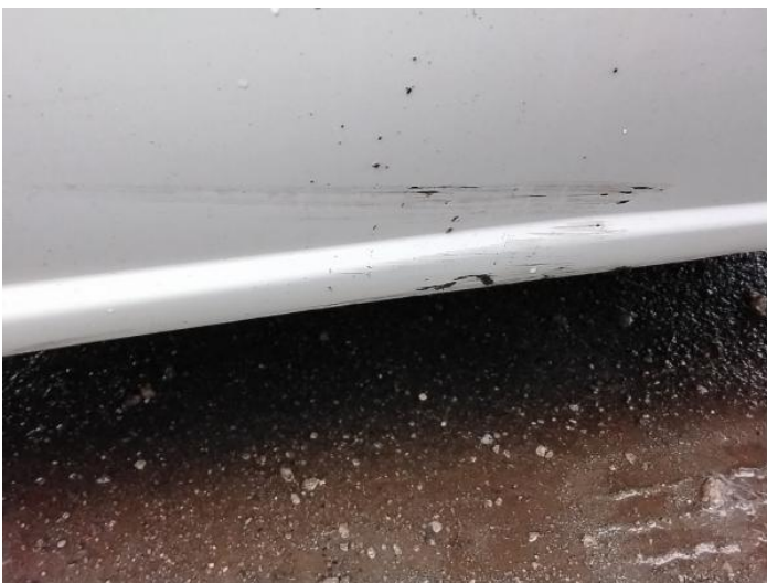
7: Qtr Panel nsr Dented With Paint Damage
