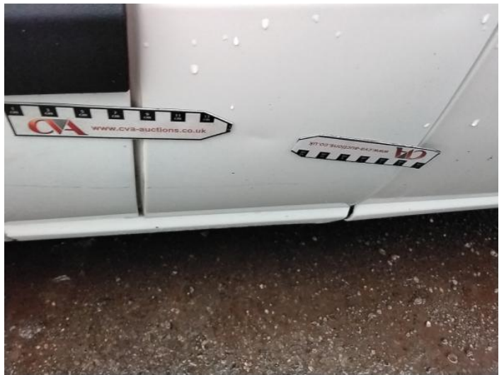
6: B Post ns Dented Over 30mm
