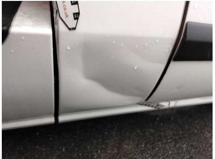
12: B Post os Dented Over 30mm
