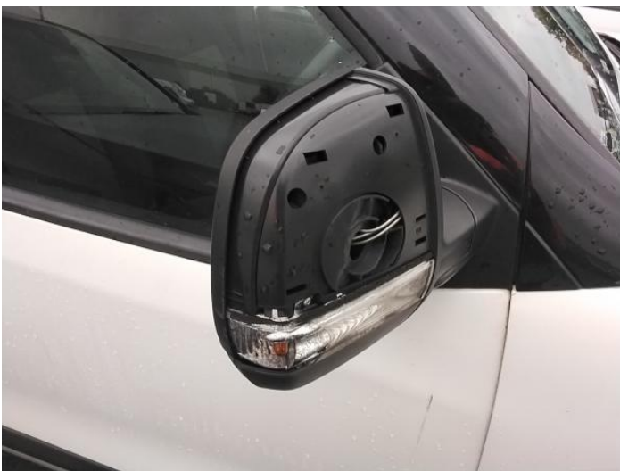
13: Door Mirror Assy osf Broken Replace
