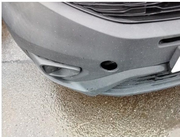
2: Bumper Front Moulding Missing Replace
