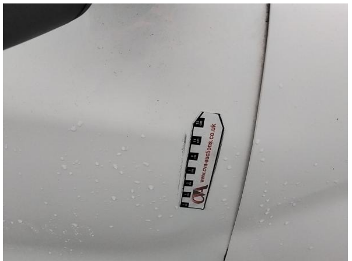
14: Door osf Scratched Over 25mm Thru Paint
