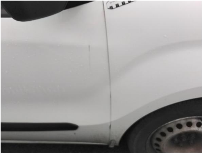
15: Door osf Dented With Paint Damage
