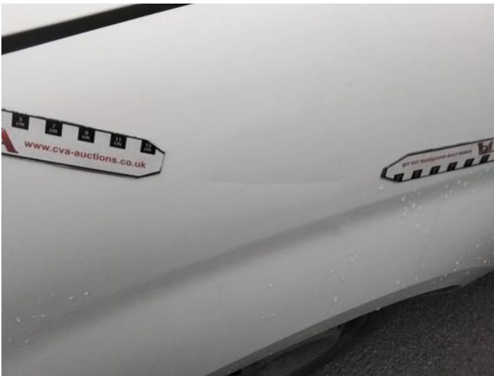
5: Wing nsf Dented With Paint Damage
