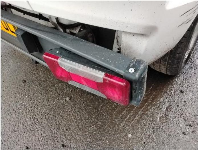
9: Bumper Rear Dented Over 30mm
