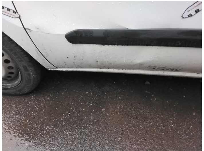
6: Door nsf Dented Over 30mm
