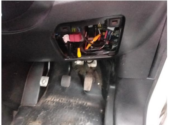
10: Fascia Panel Missing Replace
