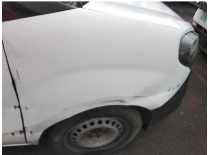
12: Wing osf Dented Over 30% Of Panel
