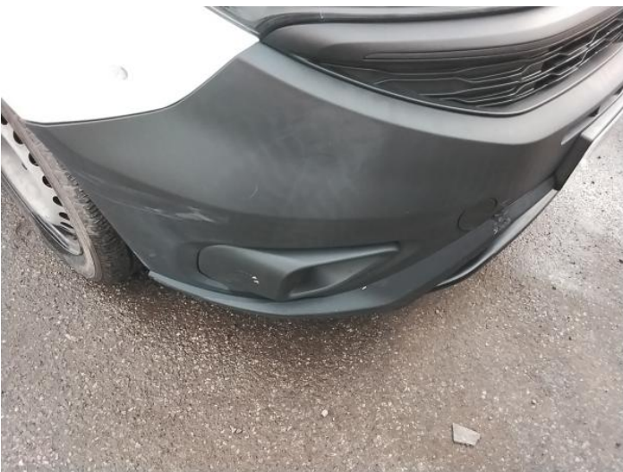
13: Bumper Front Scratched Over 100mm Thru Paint
