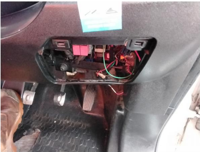
17: Fascia Panel Missing Replace
