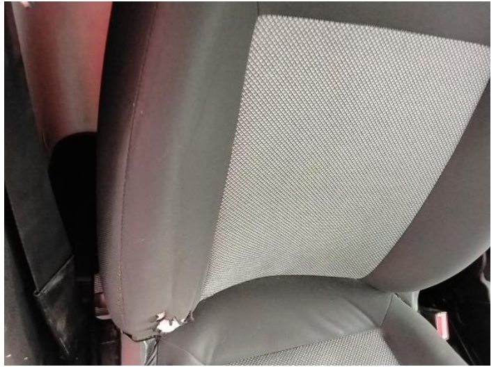
16: Seat Back Cover osf Holed Over 3mm
