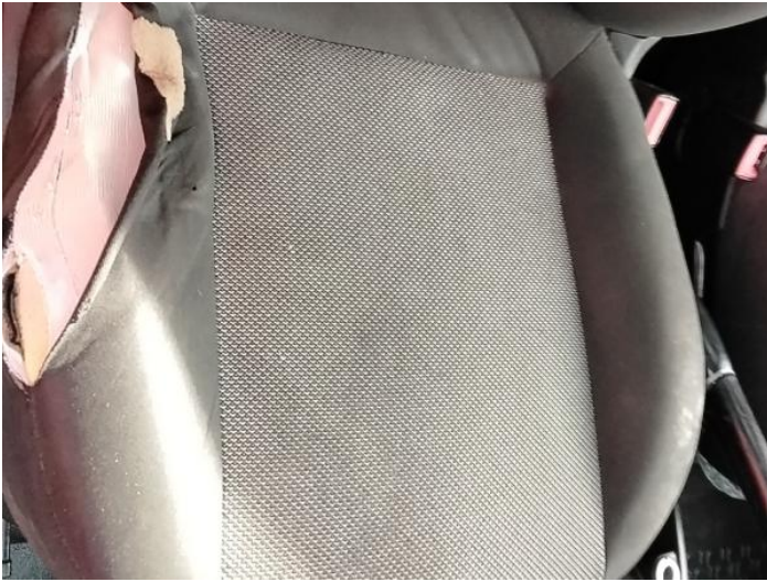
15: Seat Base Cover osf Holed Over 3mm
