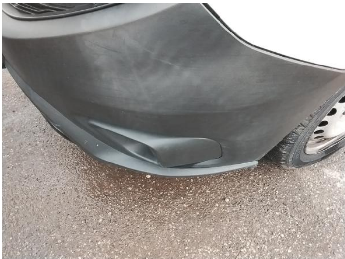
3: Bumper Front Scratched Over 100mm Thru Paint
