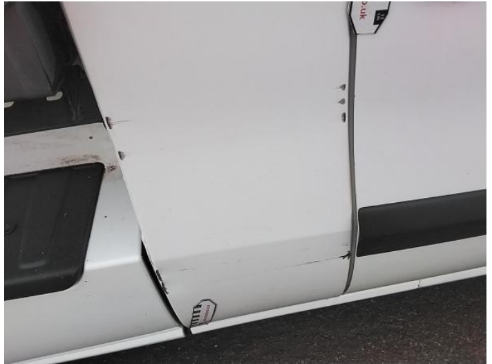
10: B Post os Dented With Paint Damage
