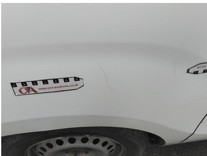
5: Wing nsf Scratched Over 25mm Thru Paint
