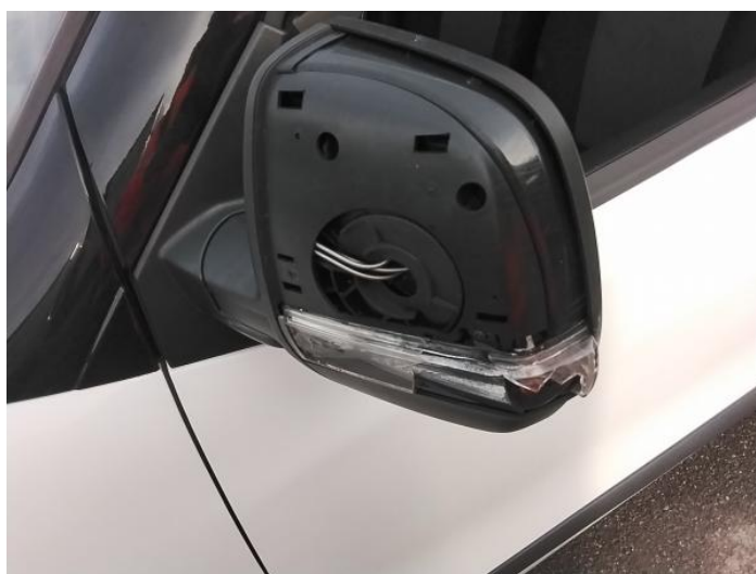
6: Door Mirror Assy nsf Broken Replace
