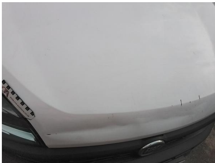
2: Bonnet Dented With Paint Damage
