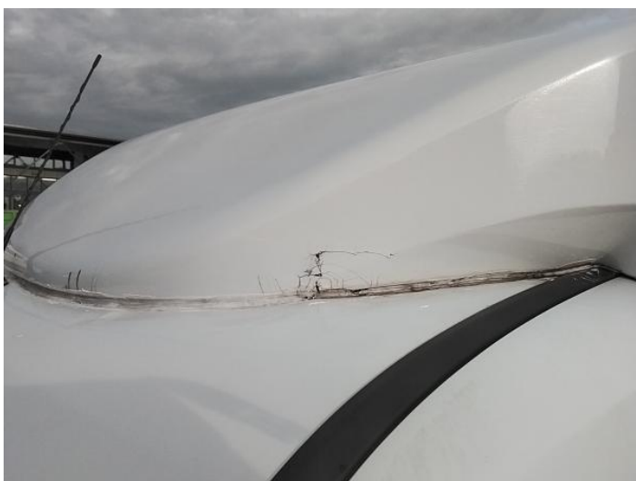
7: Qtr Panel Trim ns Broken Replace
