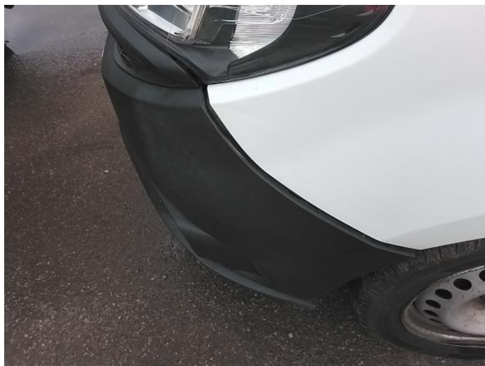
4: Bumper Front Insecure Action Required
