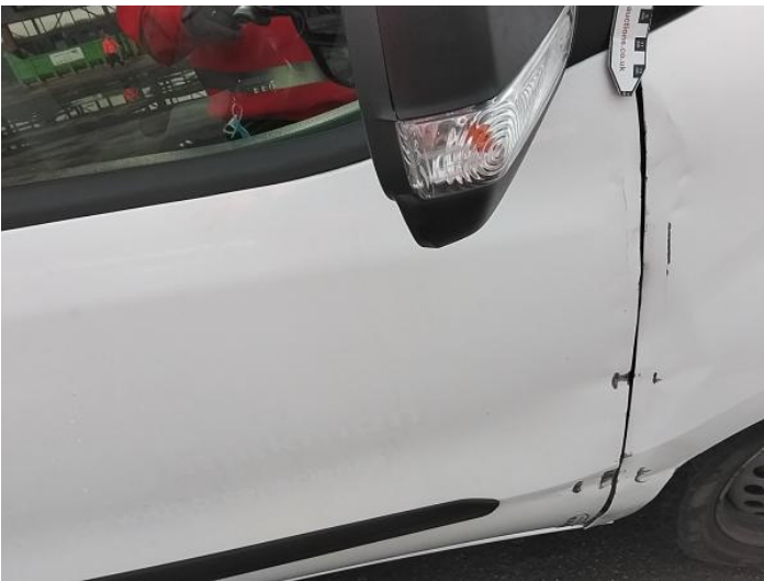
11: Door osf Dented With Paint Damage
