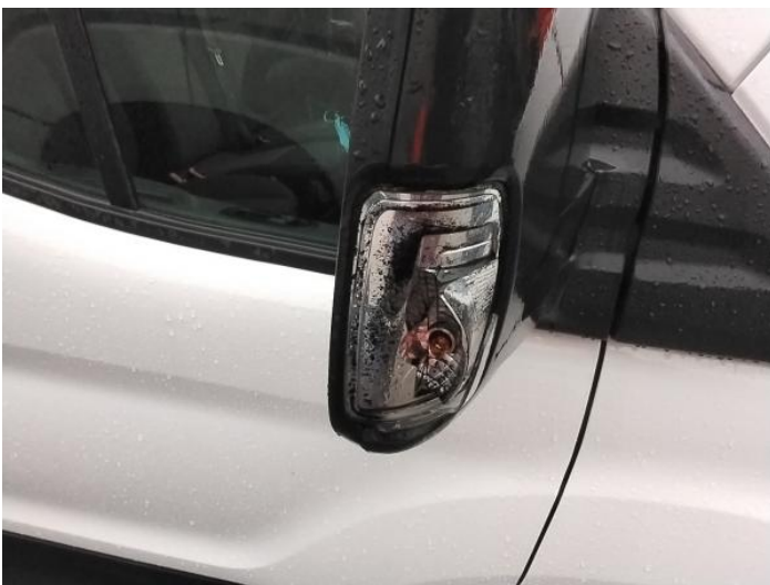
13: Door Mirror Assy osf Broken Replace
