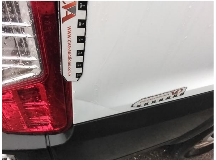
10: Qtr Panel osr Dented With Paint Damage
