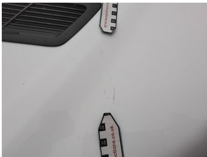
2: Bonnet Scratched Over 25mm Thru Paint
