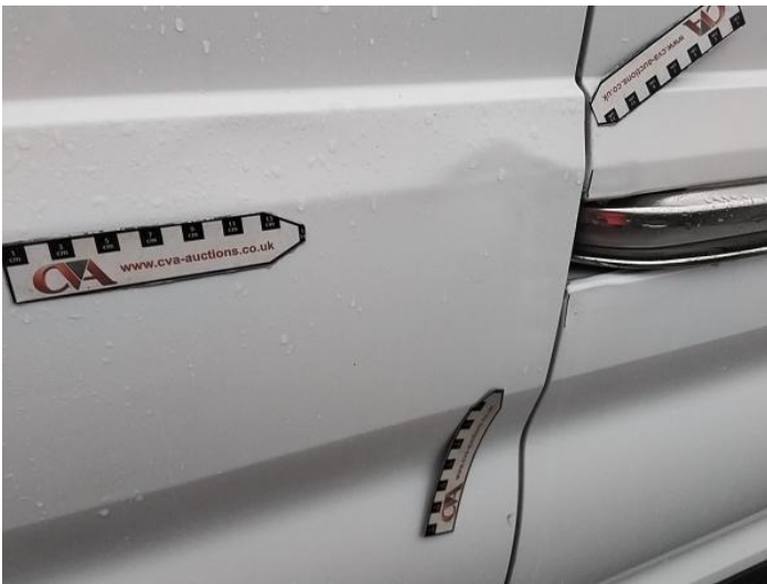
5: Qtr Panel nsr Dented Over 30mm
