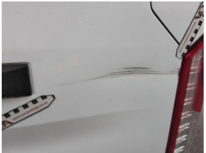
6: Qtr Panel nsr Dented With Paint Damage
