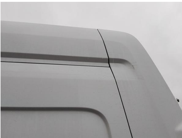
7: C Post ns Scratched Over 25mm Thru Paint
