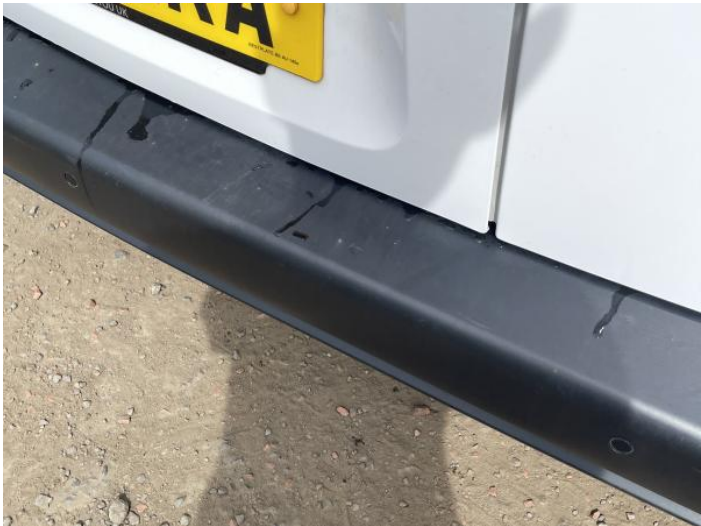
2: Bumper Rear Moulding Scuffed (Unpainted) UpTo 100mm
