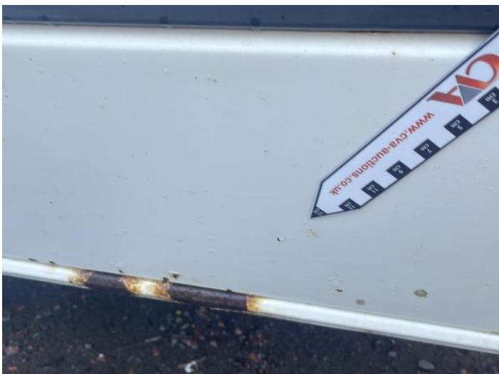
10: Sill ns Rusted Over 5mm
