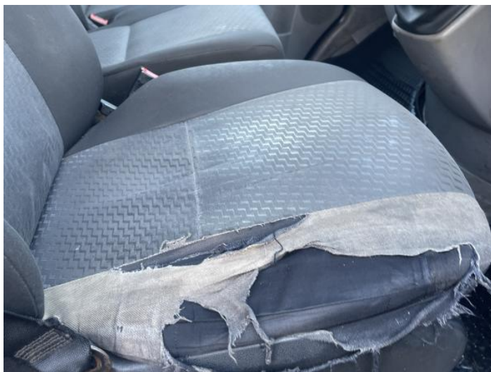
1: Seat Base Cover osf Torn Over 3mm
