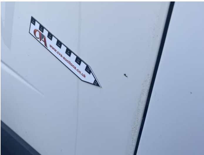
5: Door osf Dented Over 2 UpTo 10mm
