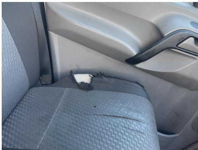
2: Seat Base Cover nsf Torn Over 3mm
