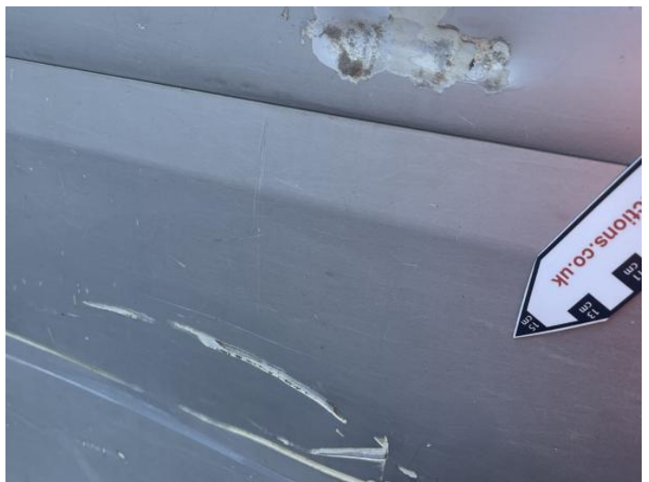
8: Qtr Panel nsr Dented Over 30mm
