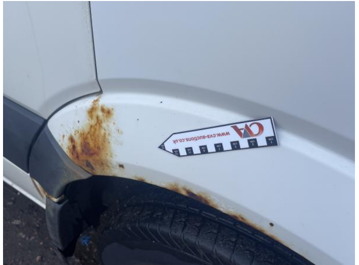
4: Wing osf Rusted Over 5mm
