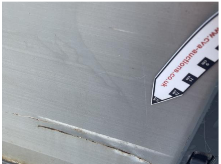
6: Qtr Panel osr Dented With Paint Damage
