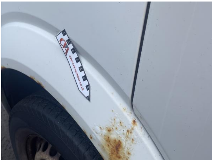
11: Wing nsf Rusted Over 5mm
