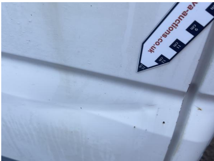
9: Door nsr Dented With Paint Damage
