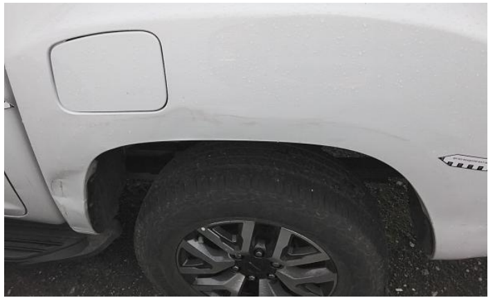
4: C Post ns Dented With Paint Damage
