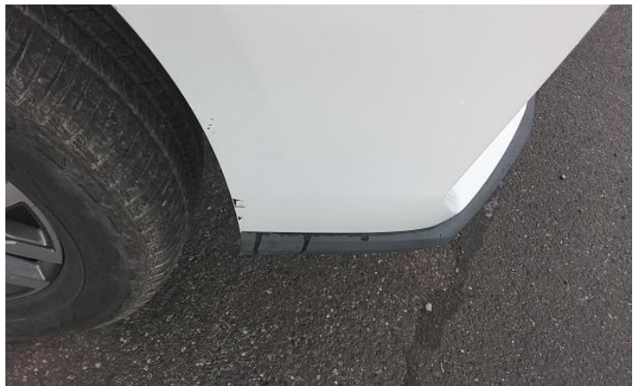
6: Qtr Panel nsr Dented With Paint Damage
