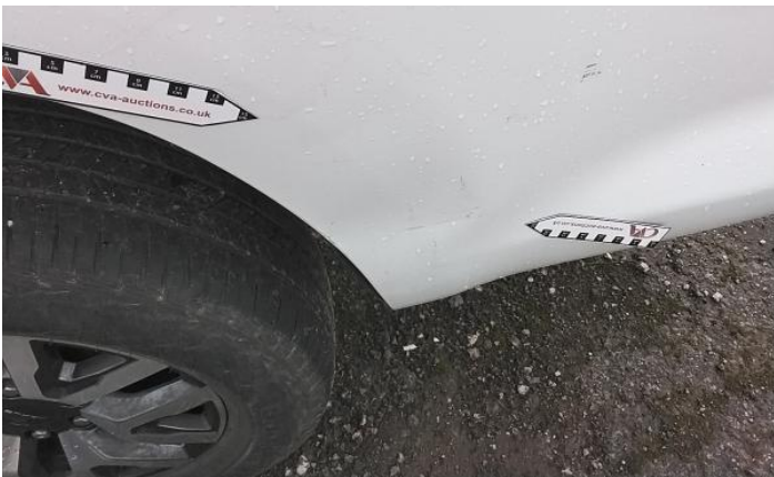
5: Qtr Panel nsr Dented With Paint Damage
