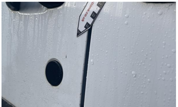
6: Qtr Panel nsr Rusted Over 5mm
