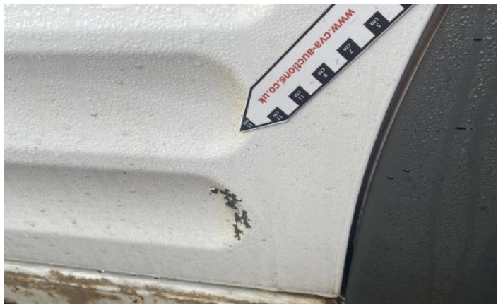
4: Sill os Rusted Over 5mm
