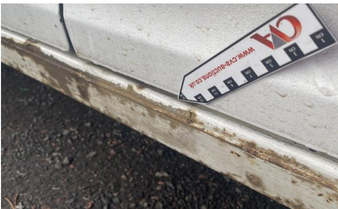
5: Qtr Panel osr Rusted Over 5mm
